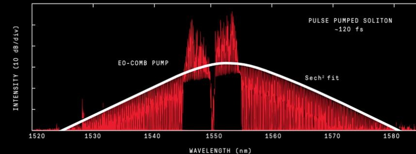
Figure showing a broad spectrum of uniformly spaced frequency comb lines generated by pulse-pumping a soliton microcomb.
