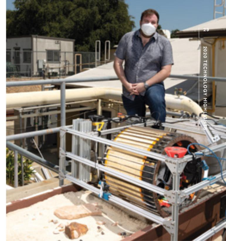
The Barefoot Rover testbed was utilized to train machine learning algorithms on different materials, surface conditions and material hydrations. Here, Jack Lightholder poses with the testbed.
