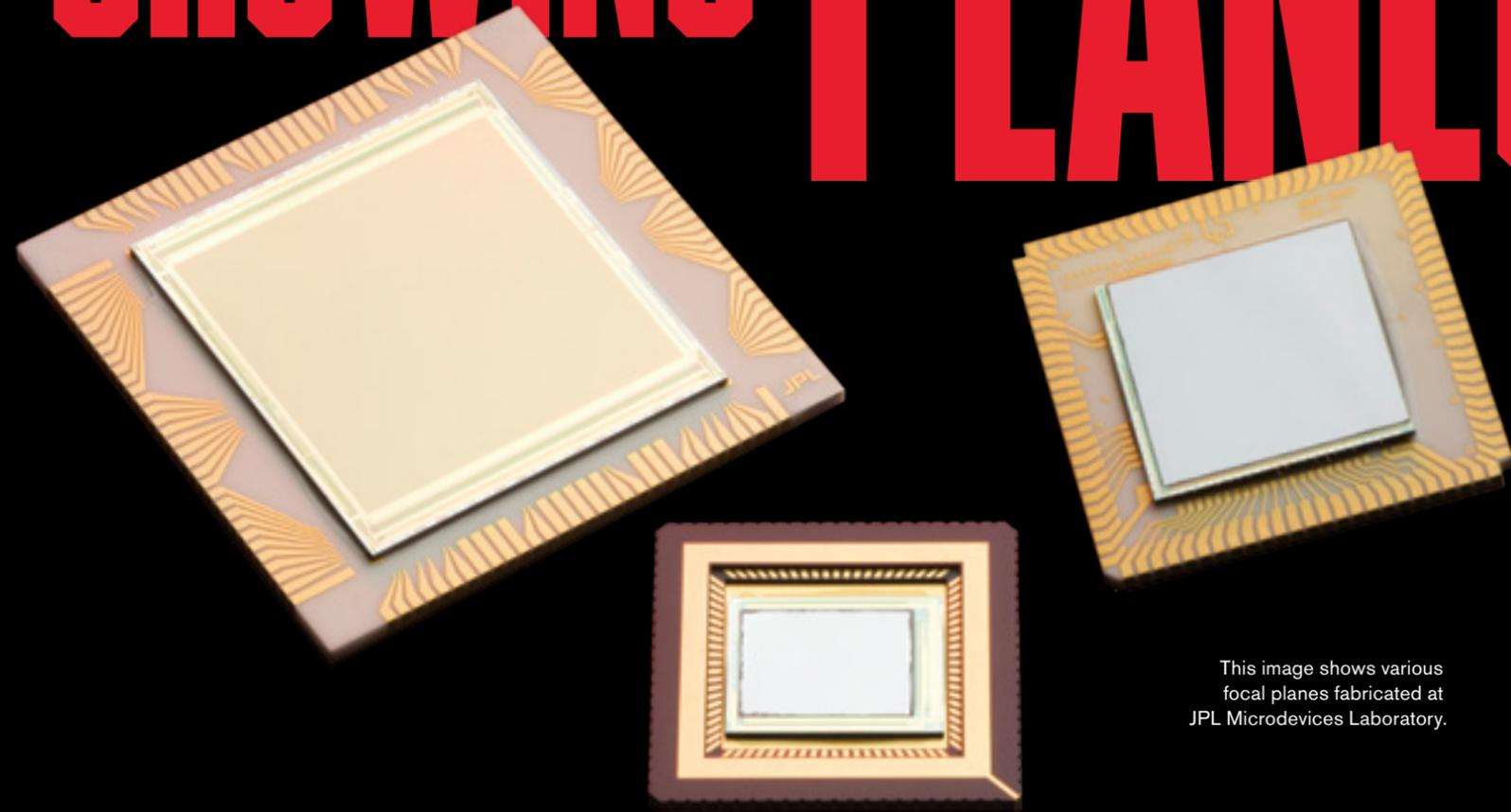
This image shows various focal planes fabricated at JPL Microdevices Laboratory.
