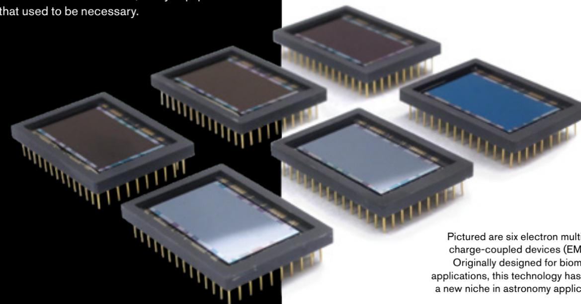
Pictured are six electron multiplying charge-coupled devices (EMCCD). Originally designed for biomedical applications, this technology has found a new niche in astronomy applications.
