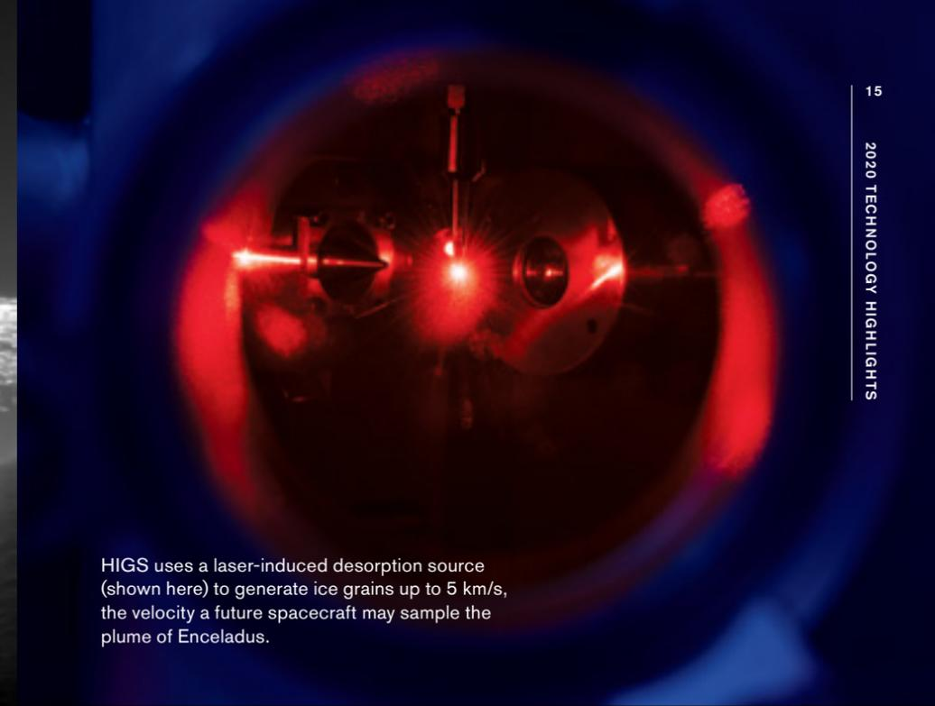
HIGS uses a laser-induced desorption source (shown here) to generate ice grains up to 5 km/s, the velocity a future spacecraft may sample the plume of Enceladus.
