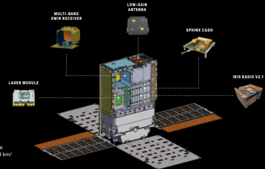
Diagram of Lunar Flashlight showing key components of this technology demonstration mission with science objectives. Lunar Flashlight will be the first SmallSat mission to use lasers to look for ice on the Moon. The selected orbits allow the spacecraft to scan 2.28 km/second on average, corresponding to 4.4 seconds of integration time every 10 km.
