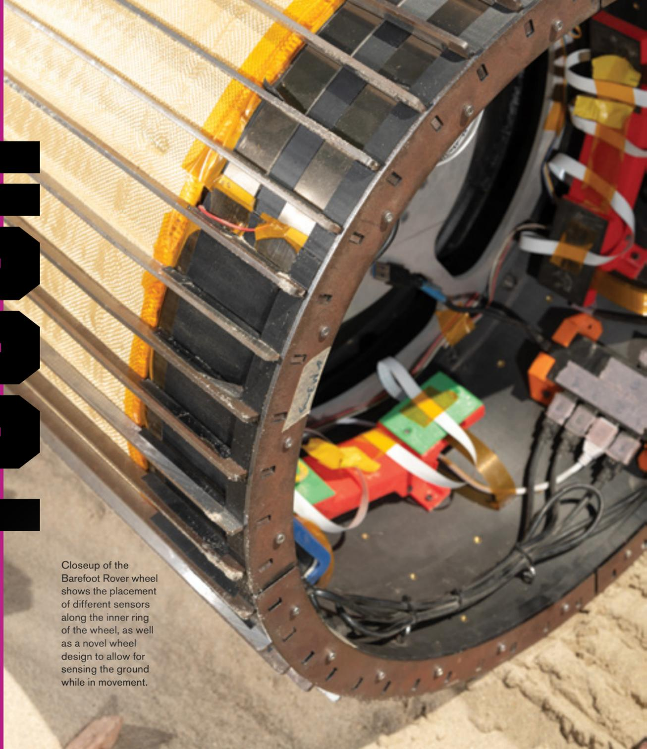
Closeup of the Barefoot Rover wheel shows the placement of different sensors along the inner ring of the wheel, as well as a novel wheel design to allow for sensing the ground while in movement.
