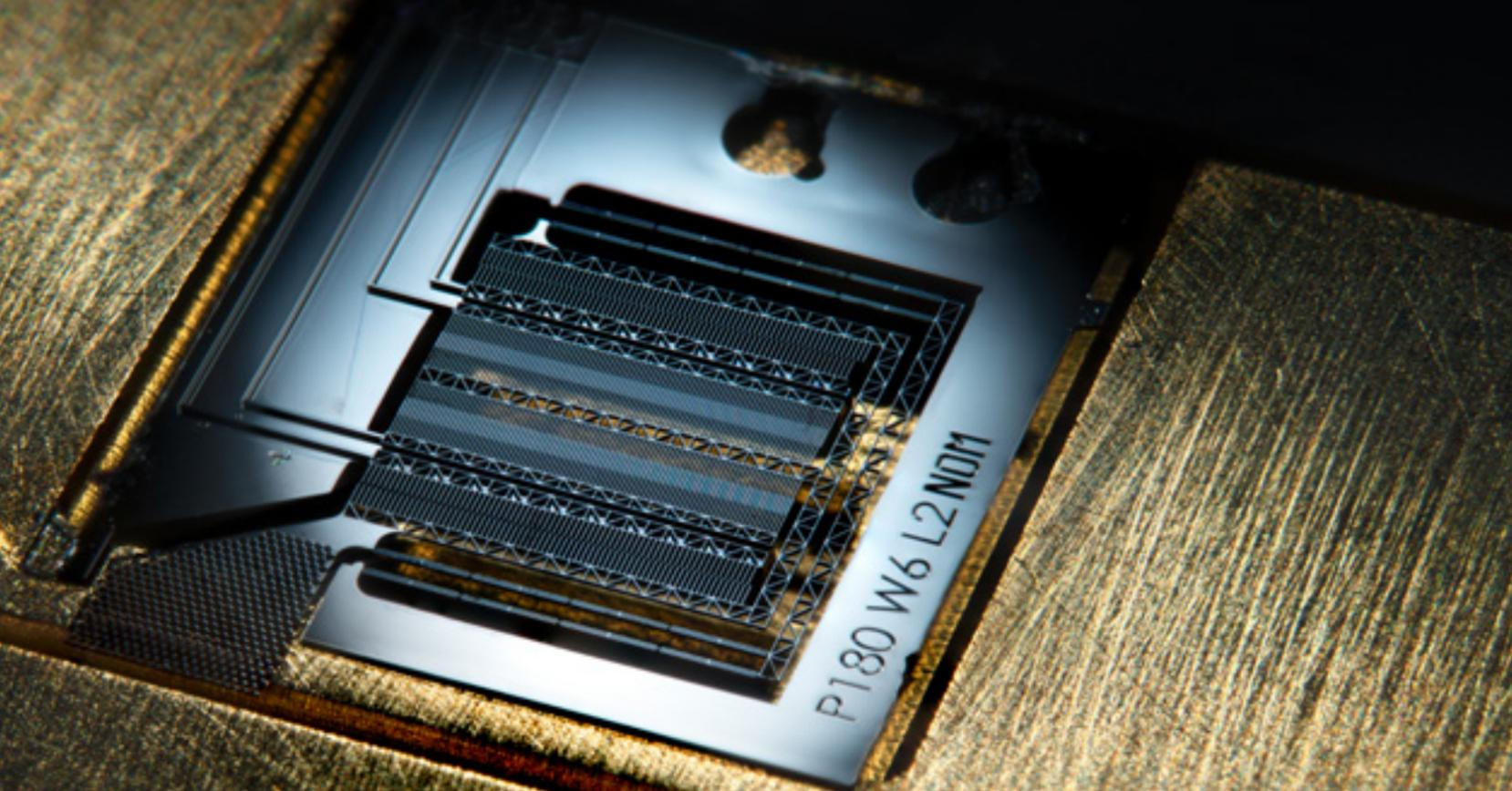
MEMs based phase shifter at submillimeter wavelengths. A silicon slab is actuated in and out of a waveguide, thereby controlling the phase shift.
