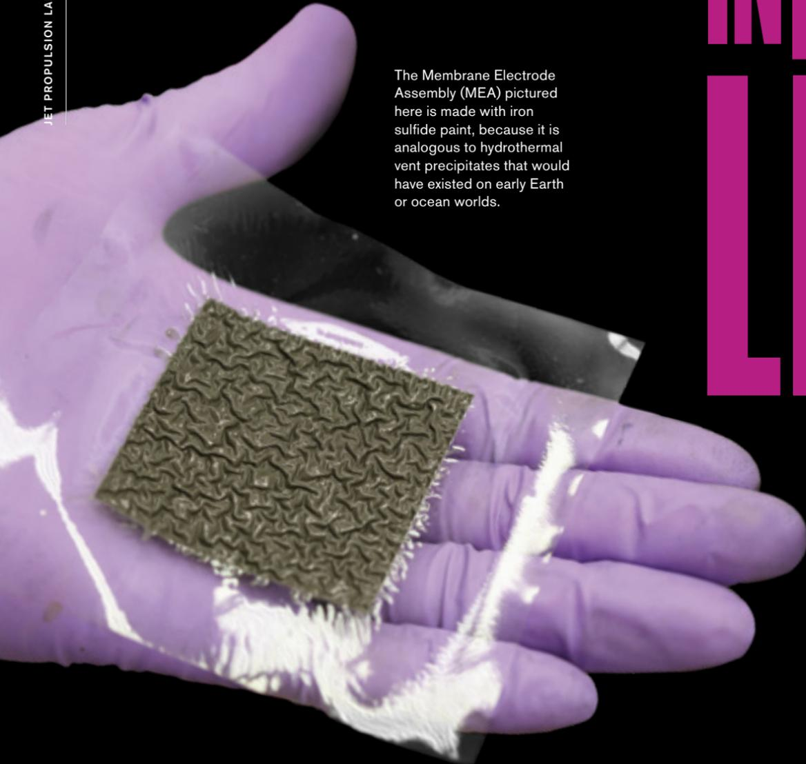
The Membrane Electrode Assembly (MEA) pictured here is made with iron sulfide paint, because it is analogous to hydrothermal vent precipitates that would have existed on early Earth or ocean worlds.
