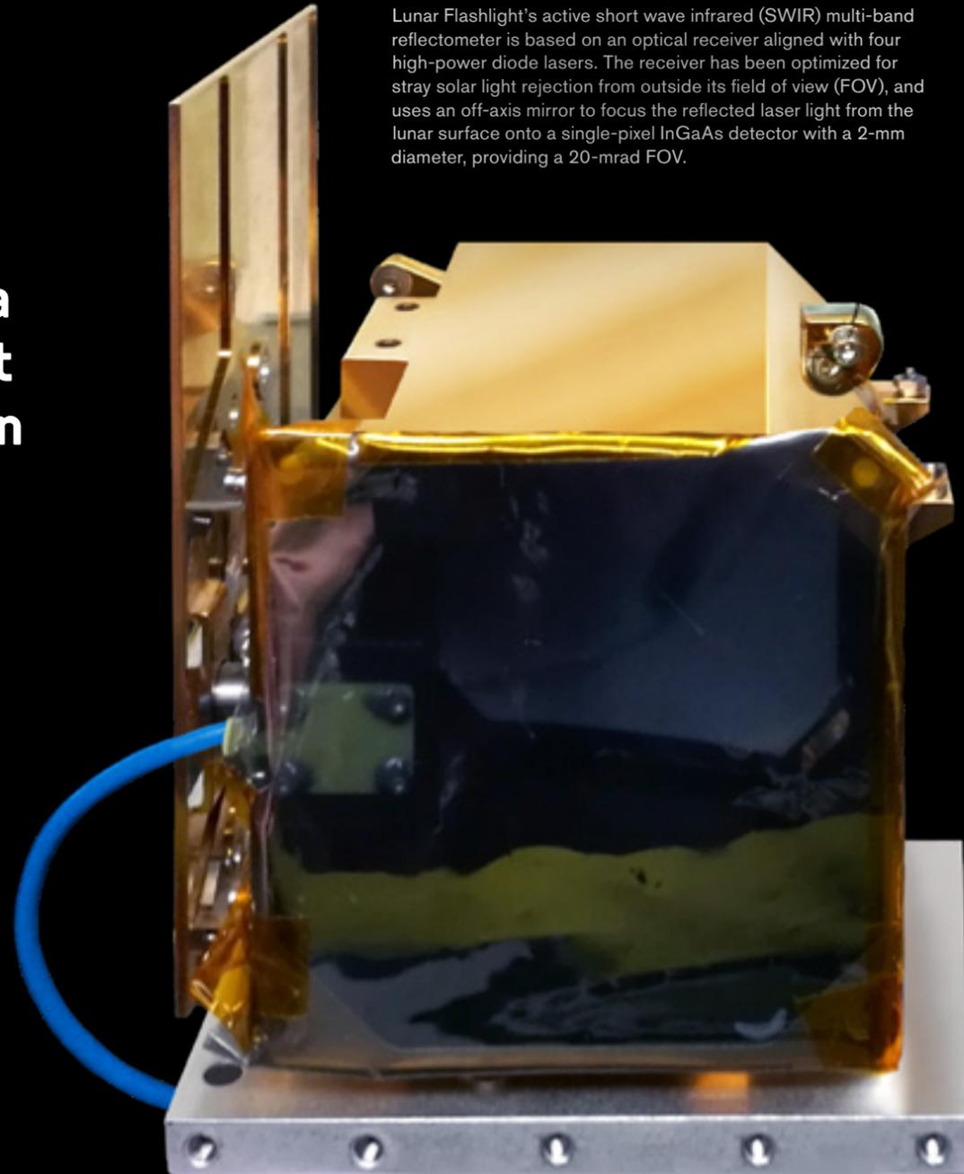
Lunar Flashlight's active short wave infrared (SWIR) multi-band reflectometer is based on an optical receiver aligned with four high-power diode lasers. The receiver has been optimized for stray solar light rejection from outside its field of view (FOV), and uses an off-axis mirror to focus the reflected laser light from the lunar surface onto a single-pixel InGaAs detector with a 2-mm diameter, providing a 20-mrad FOV.
