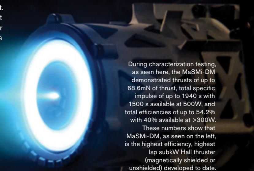
During characterization testing, as seen here, the MaSMi-DM demonstrated thrusts of up to 68.6mN of thrust, total specific impulse of up to 1940 s with 1500 s available at 500W, and total efficiencies of up to 54.2% with 40% available at >300W. These numbers show that MaSMi-DM, as seen on the left, is the highest efficiency, highest Isp subkW Hall thruster (magnetically shielded or unshielded) developed to date.
