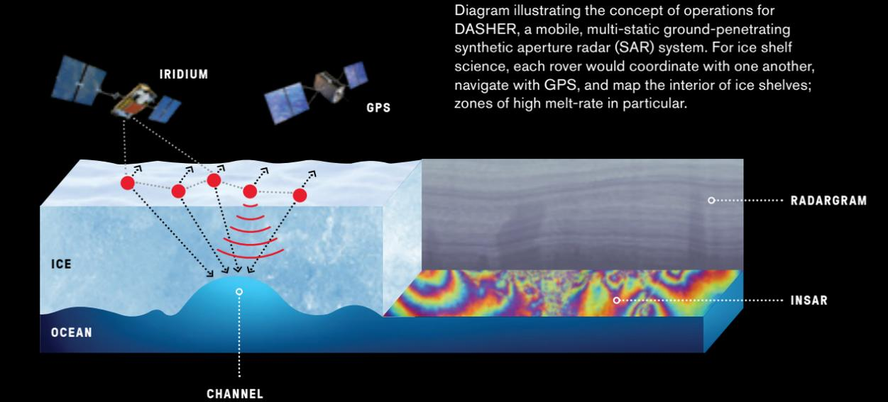
Diagram illustrating the concept of operations for DASHER, a mobile, multi-static ground-penetrating synthetic aperture radar (SAR) system. For ice shelf science, each rover would coordinate with one another, navigate with GPS, and map the interior of ice shelves; zones of high melt-rate in particular.
