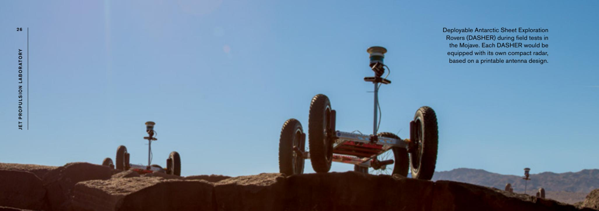
Deployable Antarctic Sheet Exploration Rovers (DASHER) during field tests in the Mojave. Each DASHER would be equipped with its own compact radar, based on a printable antenna design.
