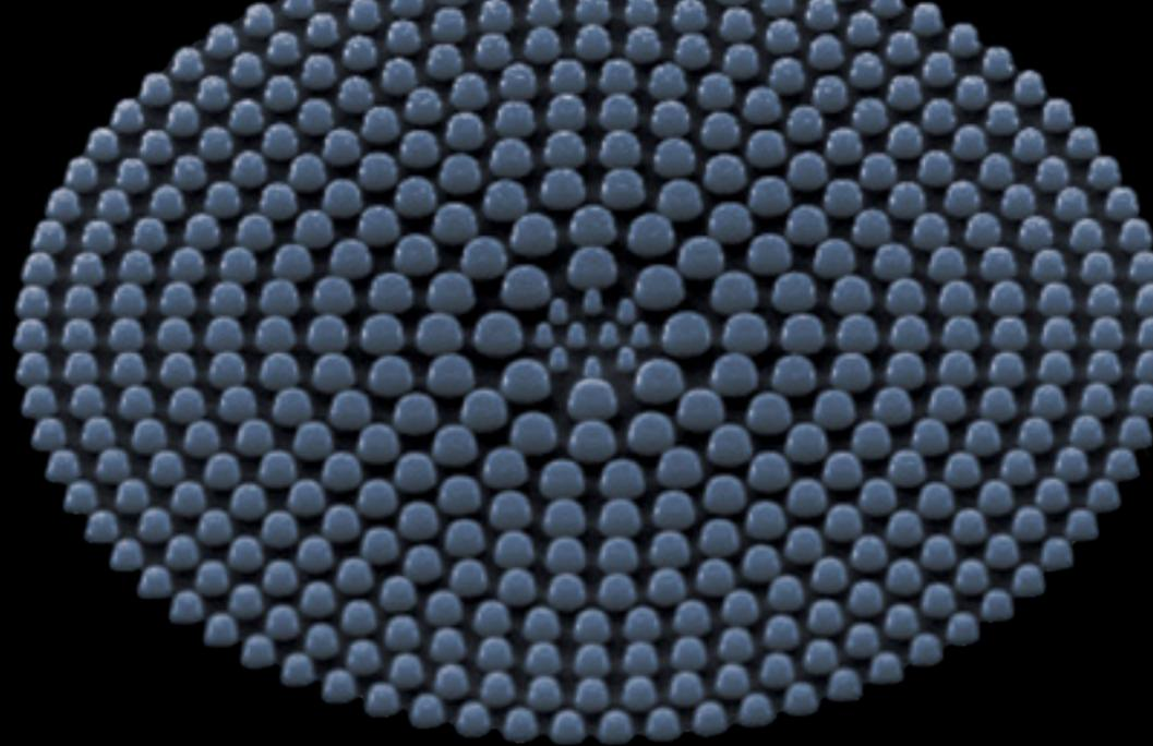
**METALENS ETCHED DIRECTLY ON TO THE DETECTOR SURFACE CONCENTRATES THE LIGHT THE SENSOR RECEIVES: ENABLING THE SYSTEM TO CAPTURE MORE DETAIL EVEN WHILE OPERATING AT HIGHER TEMPERATURES.**
