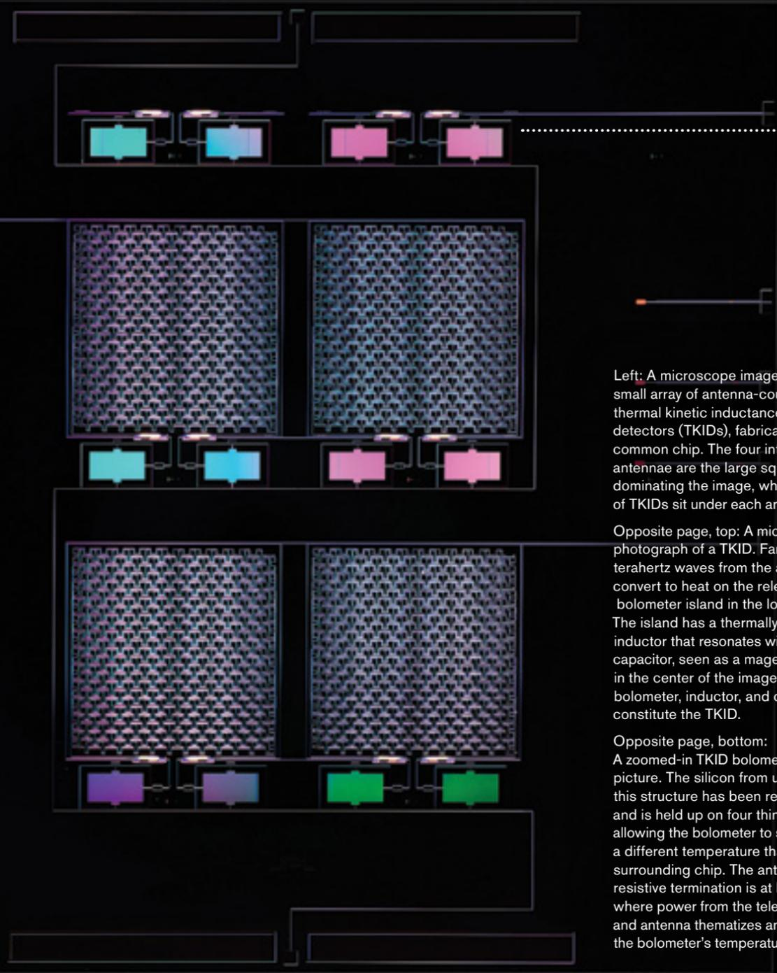
Left: A microscope image of a small array of antenna-coupled thermal kinetic inductance detectors (TKIDs), fabricated on a common chip. The four integrated antennae are the large squares dominating the image, while pairs of TKIDs sit under each antenna.
