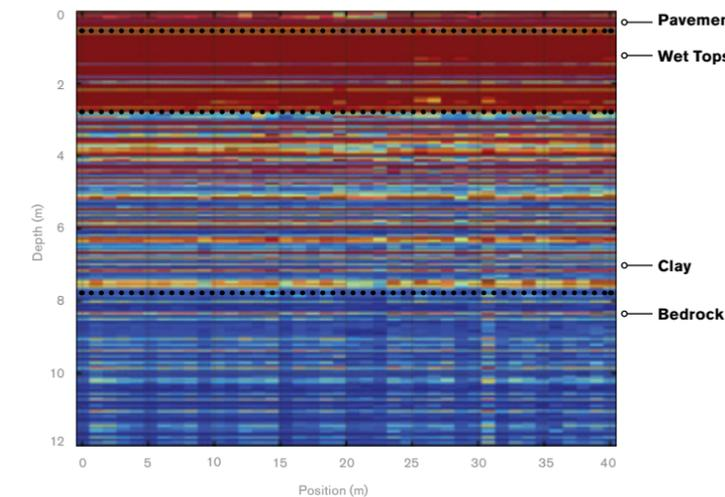
Prototype ground-penetrating radar product measuring the sub-surface beneath a road at JPL.
