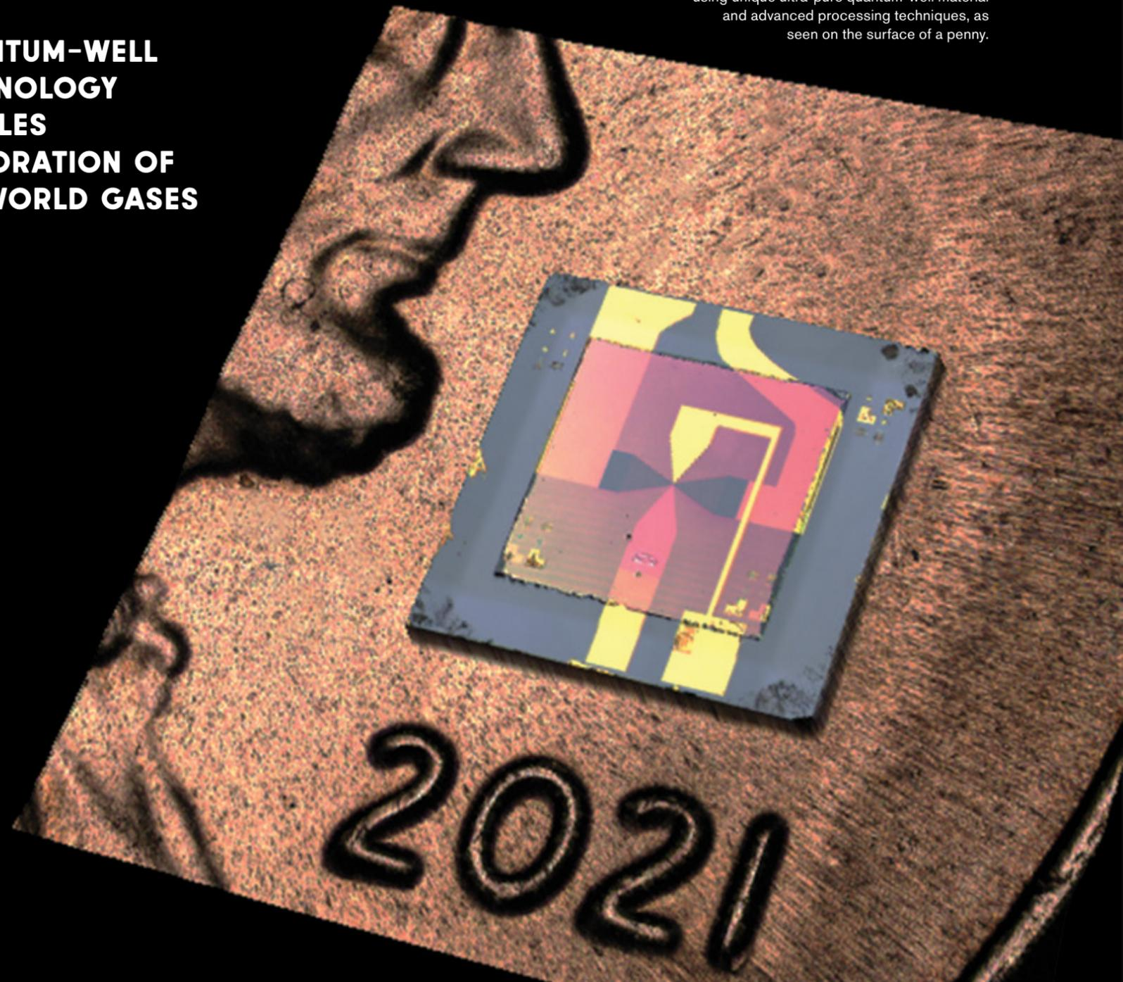
The tiny TACIT detector chip, fabricated using unique ultra-pure quantum-well material and advanced processing techniques, as seen on the surface of a penny.
