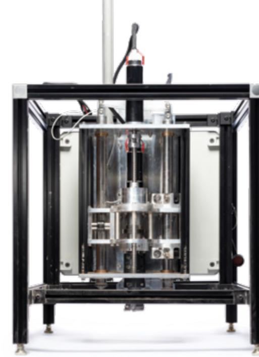
A testbed for the abrading drill bit.
