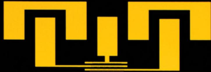
A Surface Acoustic Wave diffraction grating with a series of gold electrodes that are only 5.5 micrometers in length. The entire device is only a few hundred micrometers in length, comparable to the 100 micrometer diameter of a human hair.
