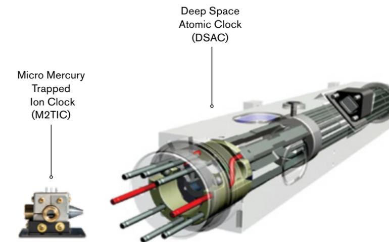
The clock trap package of the micro clock compared to that of the existing DSAC clock, a reduction of more than 10-fold in size.
