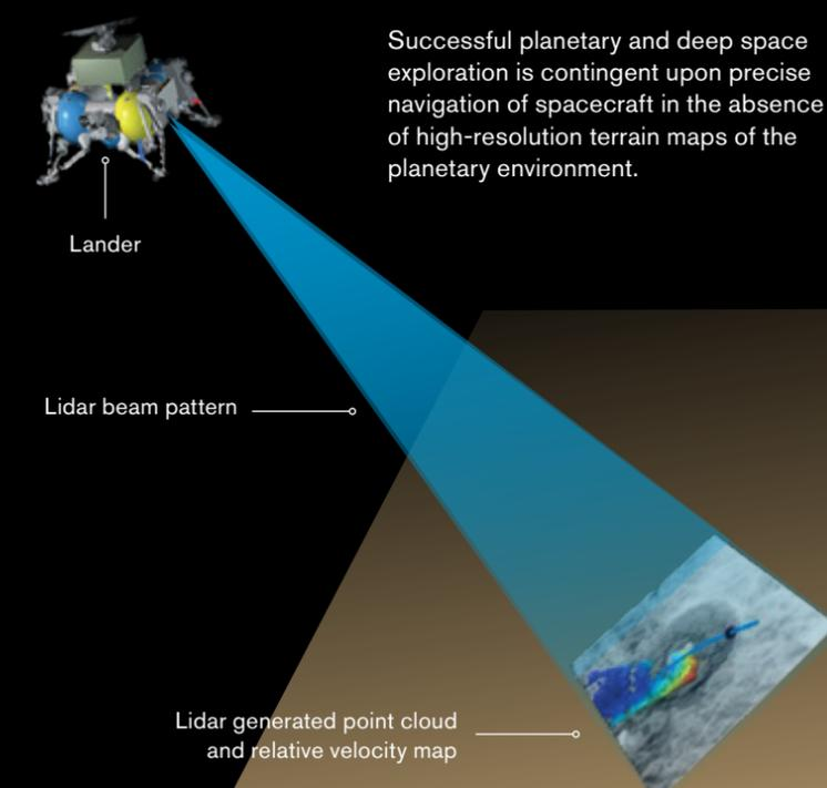
Successful planetary and deep space exploration is contingent upon precise navigation of spacecraft in the absence of high-resolution terrain maps of the planetary environment.
