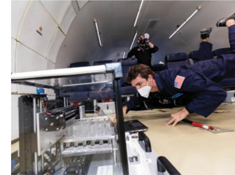
than four hours. In addition to examining dangerous germs,  $\mu$ Titan can also evaluate human DNA samples to track damage from long-term or sudden radiation exposure during spaceflight. It may also evolve to support health care in remote locations here on Earth or monitoring of the microbiome of future lunar and Martian habitats.
