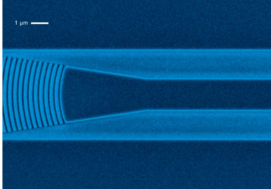
Grating coupler patterned in beta barium borate ( $\beta$ -BBO) using focused-ion-beam milling, featuring a period  $\Lambda=300$  nm and designed for operation at a wavelength of  $\lambda=460$  nm.
