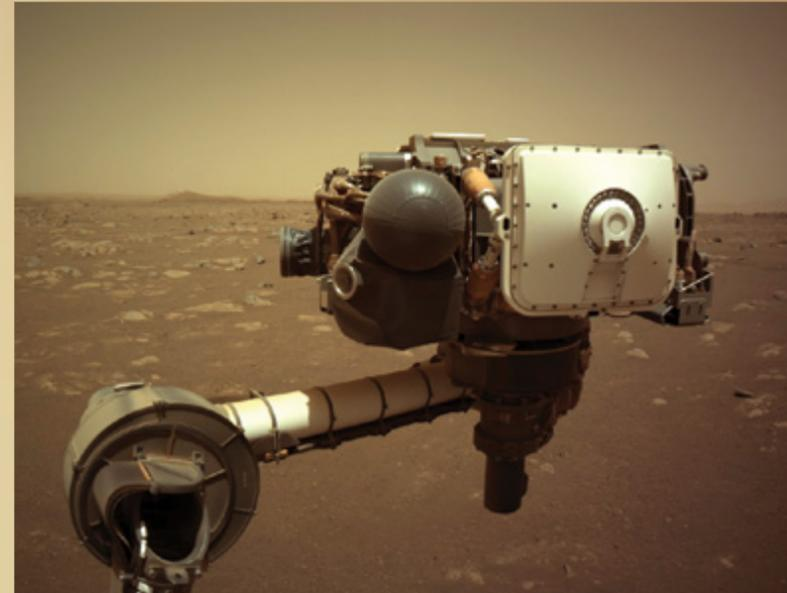
The dust removal tool mounted on the Perseverance rover on Mars.
