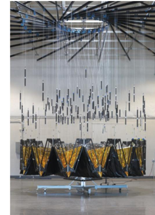
The Starshade inner disk testbed unfolds at Tendeg in Louisville, Colorado. This testbed was used to demonstrate the deployment accuracy needed for Starshade concepts.
