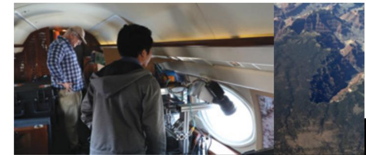
The Quakes-1 system includes 2 SWIR and 2 visible imagers that are coincident with the SAR sensor. From left to right, the system aimed out of a passenger window, a captured image, and its 3D reconstruction.
