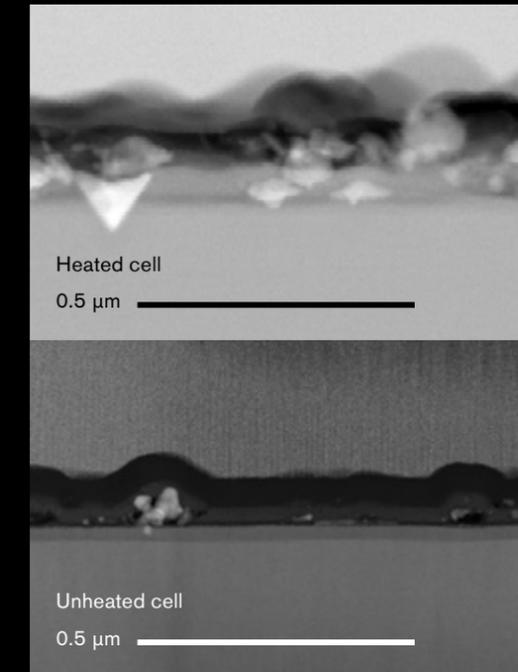
Top: Cross-sectional view of the solar cell, while heated, looking at the interface between the anti-reflective protective coating and the cell's surface. Silver melt droplets form, extending deep into the semiconductor layer.
