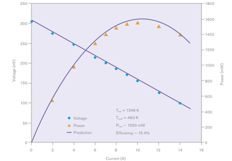
This graph shows the 15 percent thermal-to-electric conversion efficiency in an RTG enabled with JPL's new Zintl phase thermoelectric designs. Current designs have about six percent efficiency. The increase in efficiency can result in longer, more effective deep space missions.
