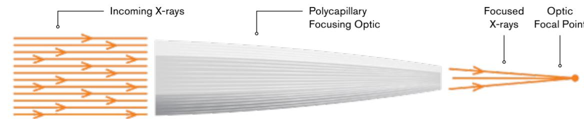
Incoming X-rays are focused by a bundle of millions of small glass capillaries, shaped to redirect the X-rays' grazing incidence to a much smaller focal spot. In this way the effective field-of-view of an X-ray detector, positioned at the focal spot, can be significantly increased.
