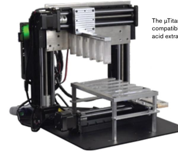
The  $\mu$ Titan—a microgravity compatible automated nucleic acid extraction system.
