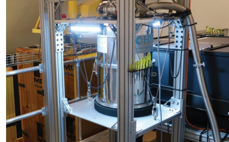
An SNSPD installed at Caltech's Mount Palomar Hale 200-inch telescope as part of the Ground Laser Receiver for the Deep Space Optical Communications (DSOC) project.
