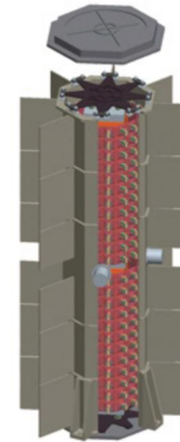
A conceptual design of an advanced RTG power source incorporating new, high-performance thermoelectric materials.
