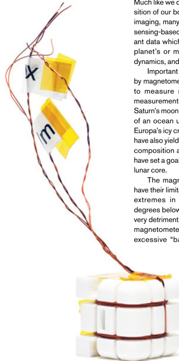
A 3-axis, 3D printed Helmholtz coil used for magnetic field modulation and field nulling.
