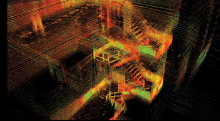
3D map generated by NeBula while traversing four flights of stairs. The map was created in real-time using onboard computation and software.
