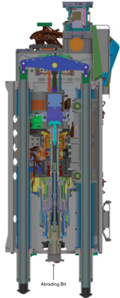
Cutaway CAD rendering of the entire drill system.
