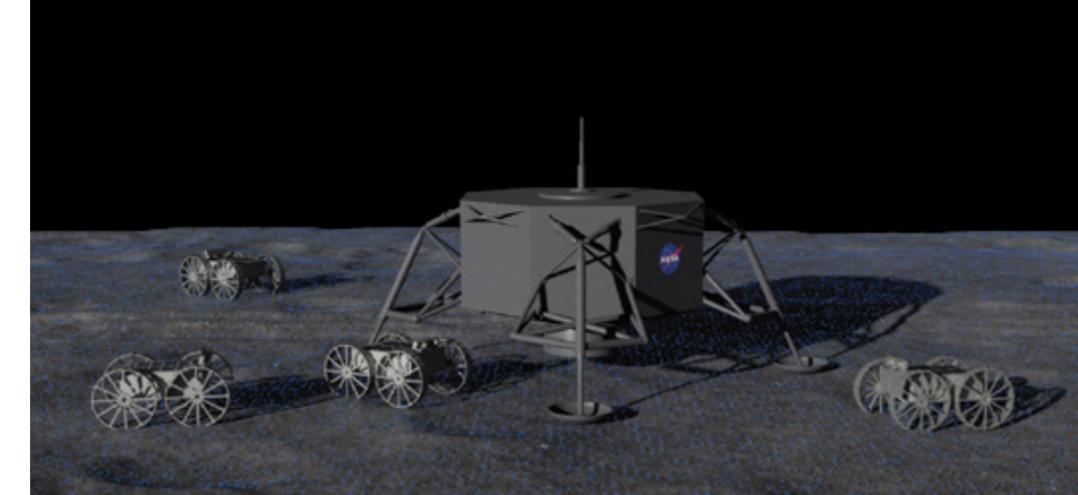
Size and mass matter greatly when exploring the solar system, especially when delivering robots to planetary surfaces. A new breed of small, autonomous scouting rovers is under development that may redefine how we explore lunar and planetary terrain. These machines are smaller (about the size of a shoebox), faster, more nimble, and less expensive than the larger “parent” rovers and landers they are designed to augment.
