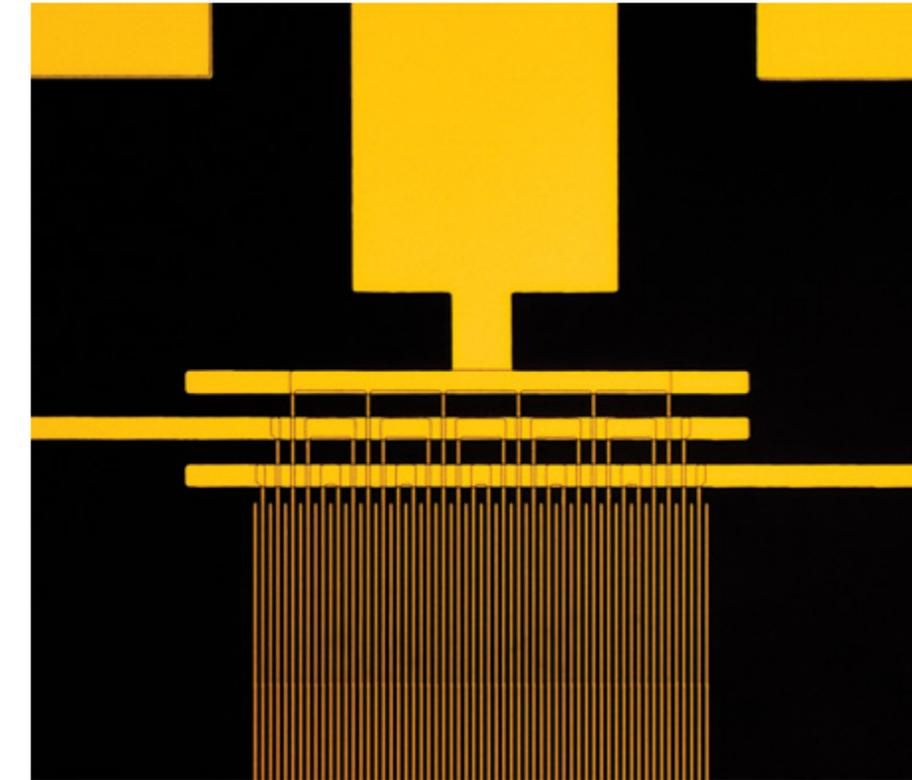
An optical image of a tunable surface acoustic wave transducers used for tunable-pitch diffraction gratings.
