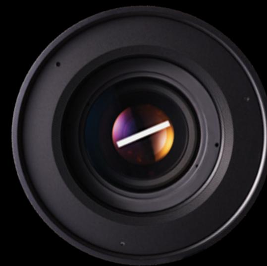
The iris in this lens has been replaced with a strip-aperture pupil replicating the essential physics of RSA imaging.
