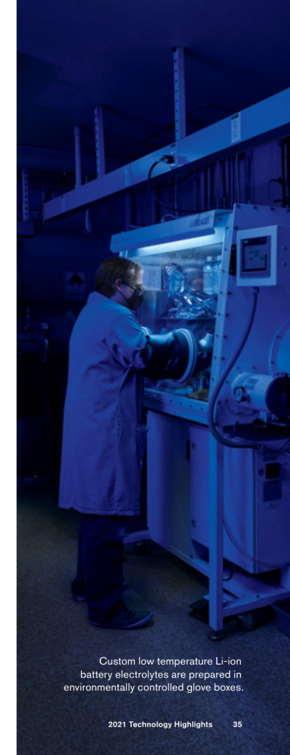
Custom low temperature Li-ion battery electrolytes are prepared in environmentally controlled glove boxes.
