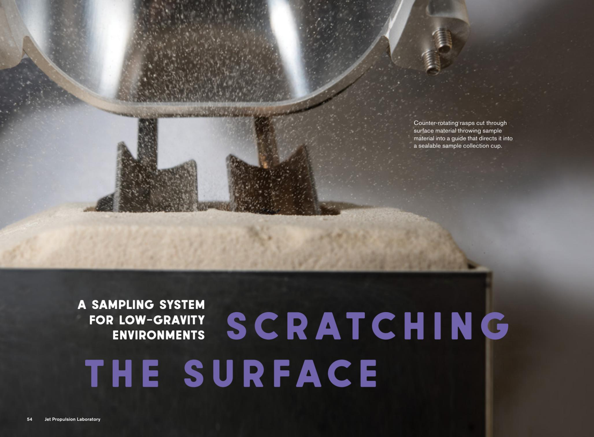
Counter-rotating rasps cut through surface material throwing sample material into a guide that directs it into a sealable sample collection cup.
