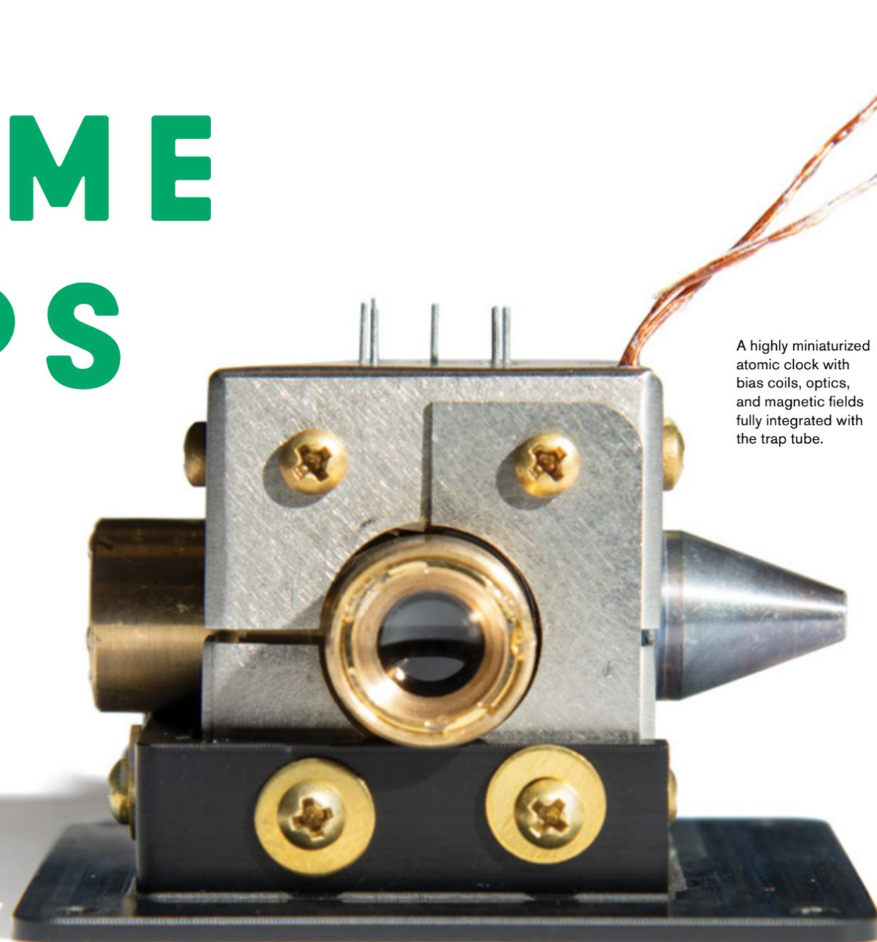
A highly miniaturized atomic clock with bias coils, optics, and magnetic fields fully integrated with the trap tube.
