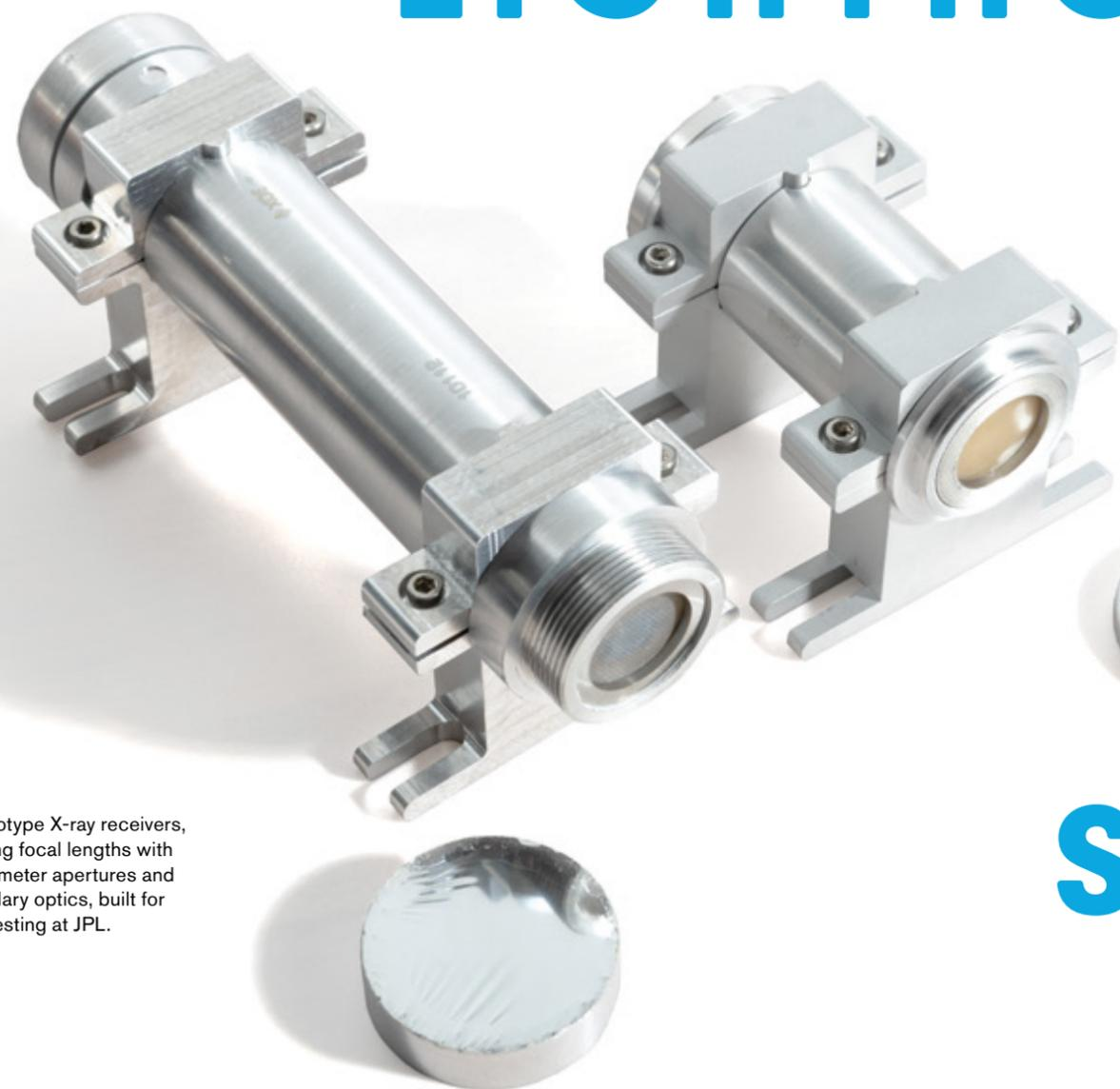
Two prototype X-ray receivers, of differing focal lengths with 2-cm diameter apertures and polycapillary optics, built for ground testing at JPL.
