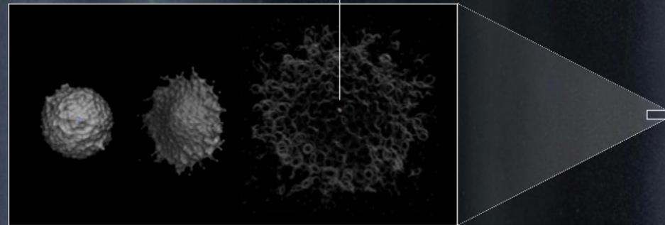
On the cover is the computer simulation of arginine amino acid encased in a 6.4 nm ice grain survives a simulated hard impact at 5 km/s. This provides quantifiable insight into future instrument design and mission parameters for hypervelocity sampling of biosignatures from ocean world atmospheres and plumes.
