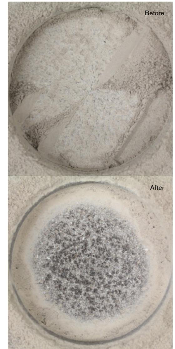
Dust removal test results, before (top) and after (bottom) being cleaned with high-pressure gas.
