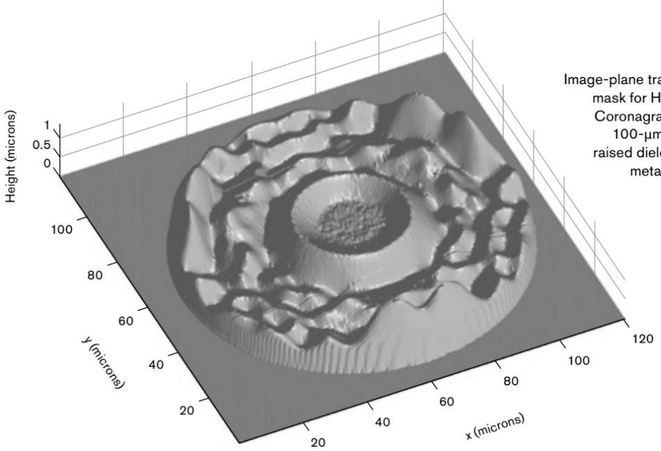
Image-plane transmitting mask for Hybrid Lyot Coronagraph (HLC), 100- $\mu$ m diameter, raised dielectric and metal on glass.
