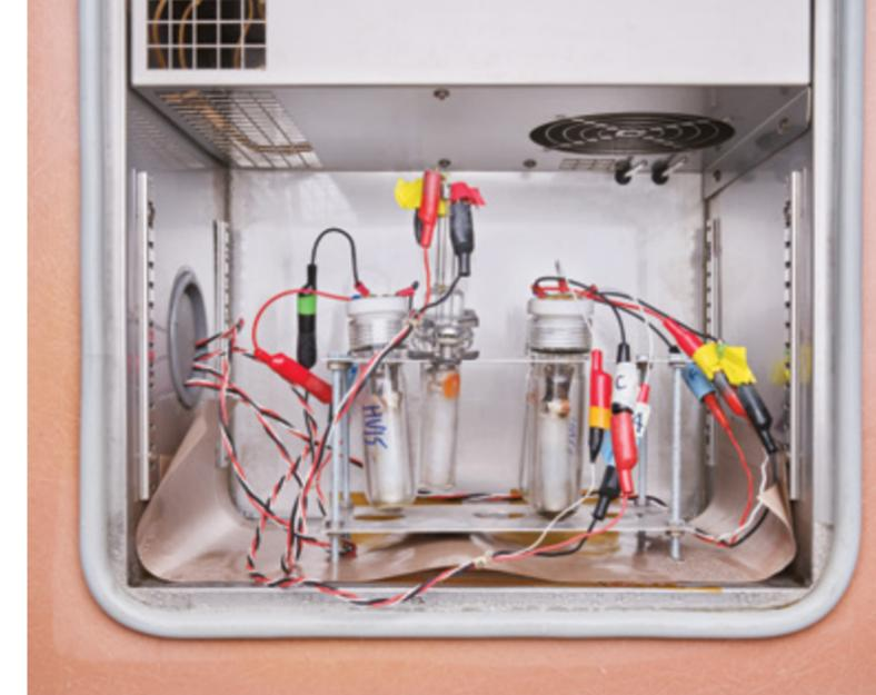
The electrochemical characteristics of electrolytes are studied in experimental 3-electrode cells.
