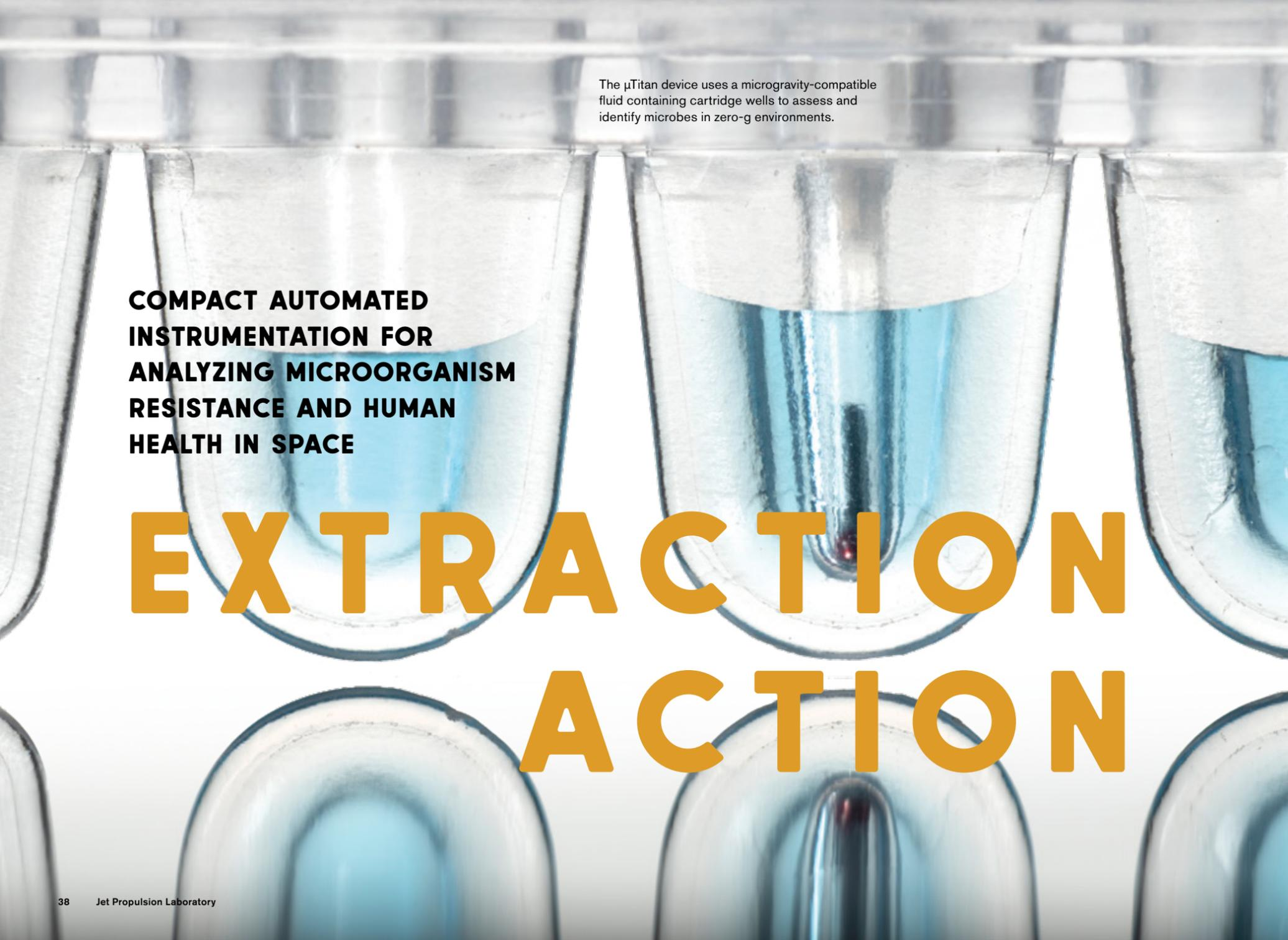
The  $\mu$ Titan device uses a microgravity-compatible fluid containing cartridge wells to assess and identify microbes in zero-g environments.
