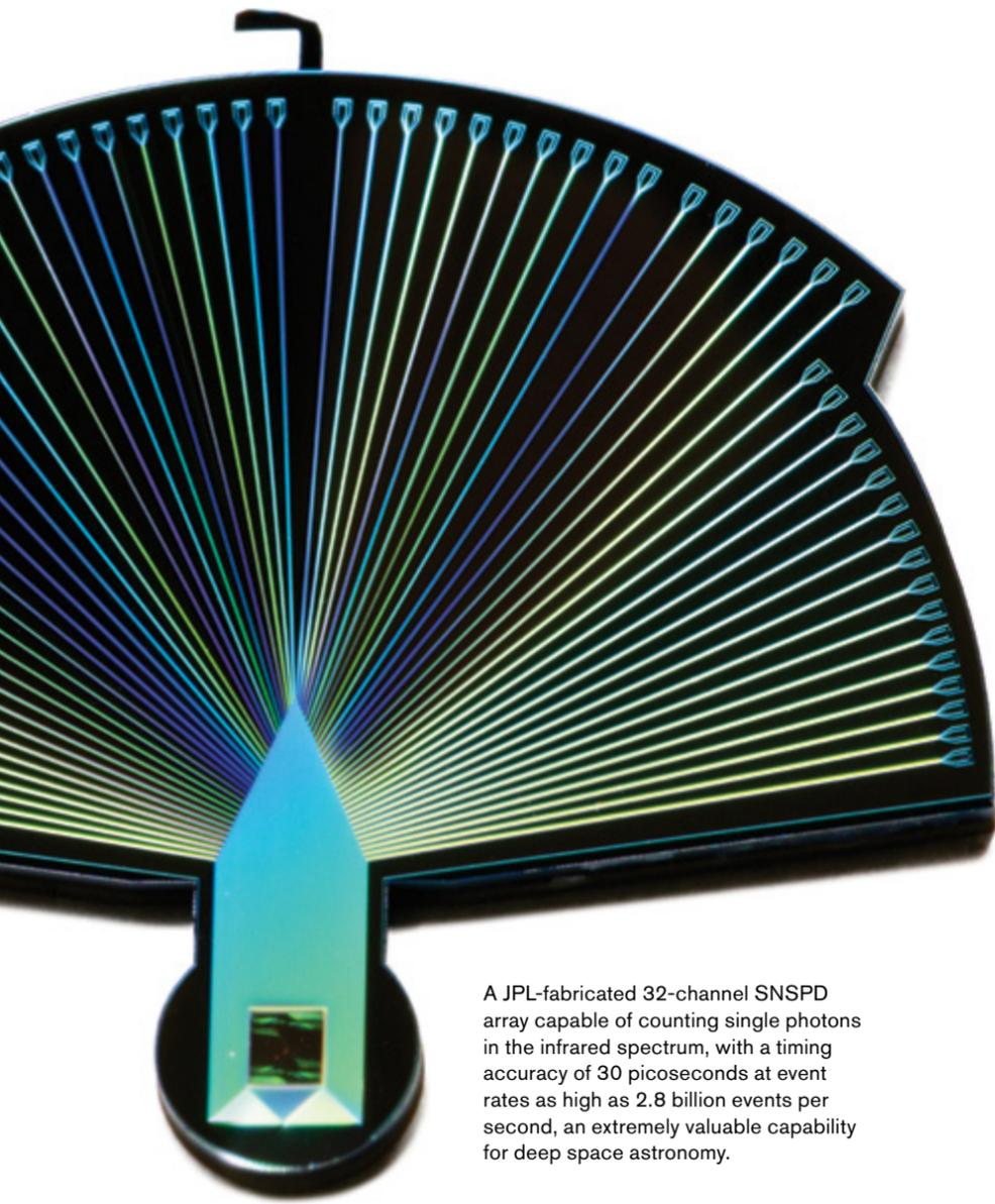
A JPL-fabricated 32-channel SNSPD array capable of counting single photons in the infrared spectrum, with a timing accuracy of 30 picoseconds at event rates as high as 2.8 billion events per second, an extremely valuable capability for deep space astronomy.
