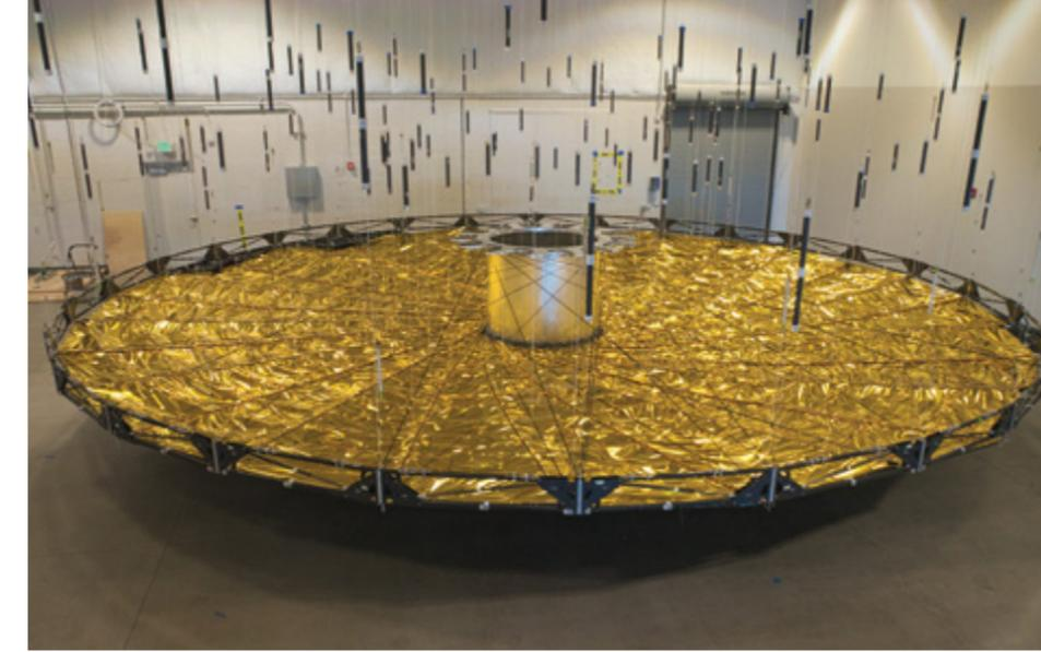
The Starshade Inner Disk System (IDS) prototype deployed in testing. The IDS is about 35 feet (10.6 meters) in diameter when deployed.
