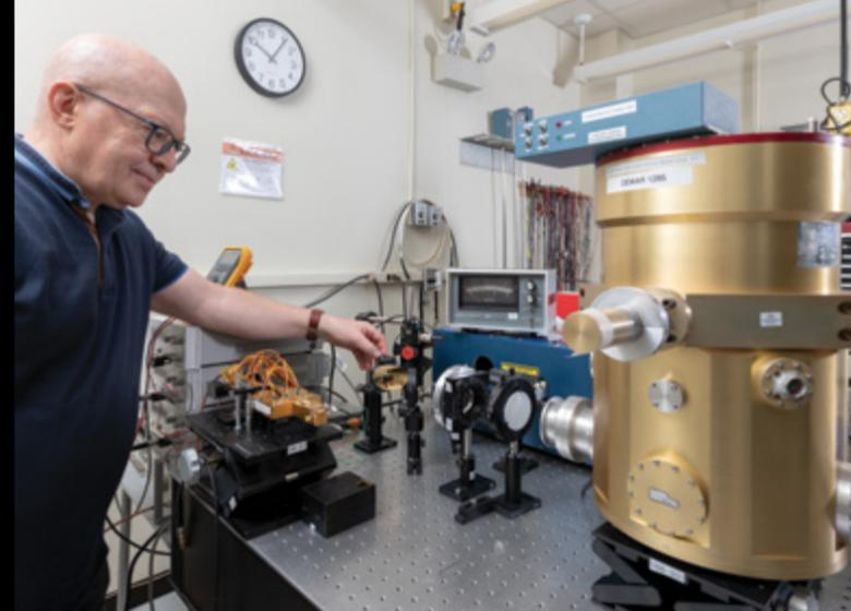
TACIT detector prototypes are tested at JPL using various radiation sources.
