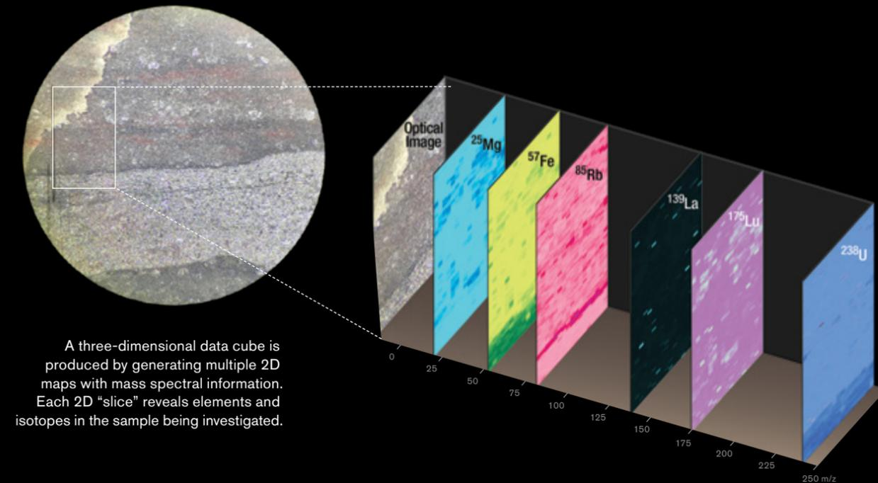
A three-dimensional data cube is produced by generating multiple 2D maps with mass spectral information. Each 2D "slice" reveals elements and isotopes in the sample being investigated.
