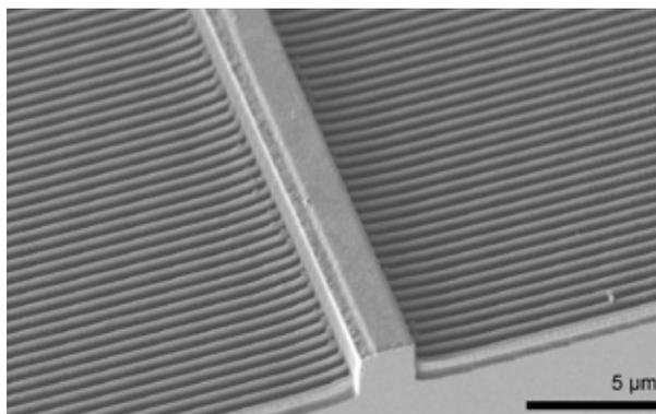
Above left: Two bars of GaSb-based lasers processed in the MDL cleanroom facility. A single bar consists of 16 individual lasers, each of which is capable of producing more than 50 mW of optical power at 2.05- $\mu\text{m}$  wavelength. Right: Scanning electron micrograph showing the structure of a DFB laser with an etched, laterally coupled diffraction grating.
