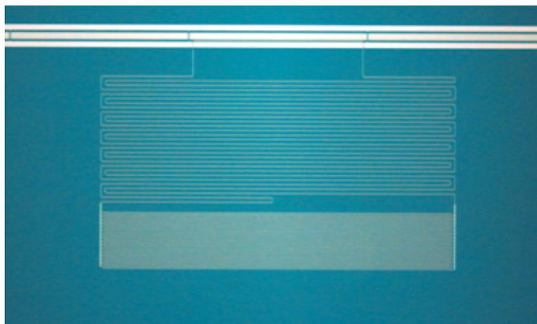
Low-frequency KID resonator consisting of a superconducting NbTiN meandered inductor (top) and an interdigitated capacitor (bottom) coupled to a coplanar waveguide feedline (running across the top).
