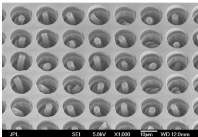
Carbon nanotube emitters integrated with extraction gate electrodes using a MDL-developed process.
