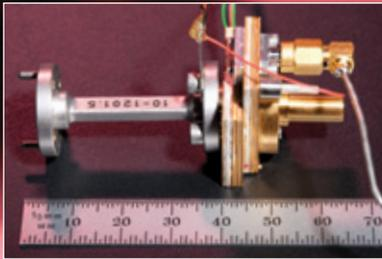
Left: A 600-GHz receiver front-end has been demonstrated that is built with the radiometer-on-a-chip technology (pictured below). This technology will allow us to make compact array receivers for future NASA missions.
