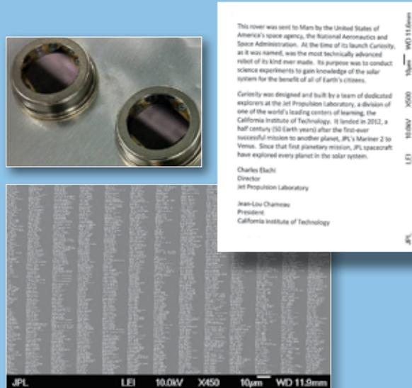
Above: SEM Micrographs of some of the over 1.2 million names and signatures and a message from the JPL director and President of Caltech contained on the two chips fabricated and packaged in MDL (pictured). The chips were attached to the MSL rover for delivery to the surface of Mars as part of NASA/JPL's outreach activities.
