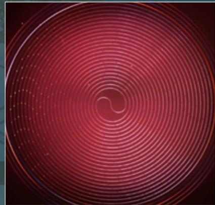
Above: The traveling-wave kinetic inductance parametric amplifier consists of a 1-meter section of NbTiN coplanar waveguide transmission line, compactly arranged in a double spiral. The nonlinearity of the line allows a weak signal tone to draw power from a strong pump tone, producing gain.
