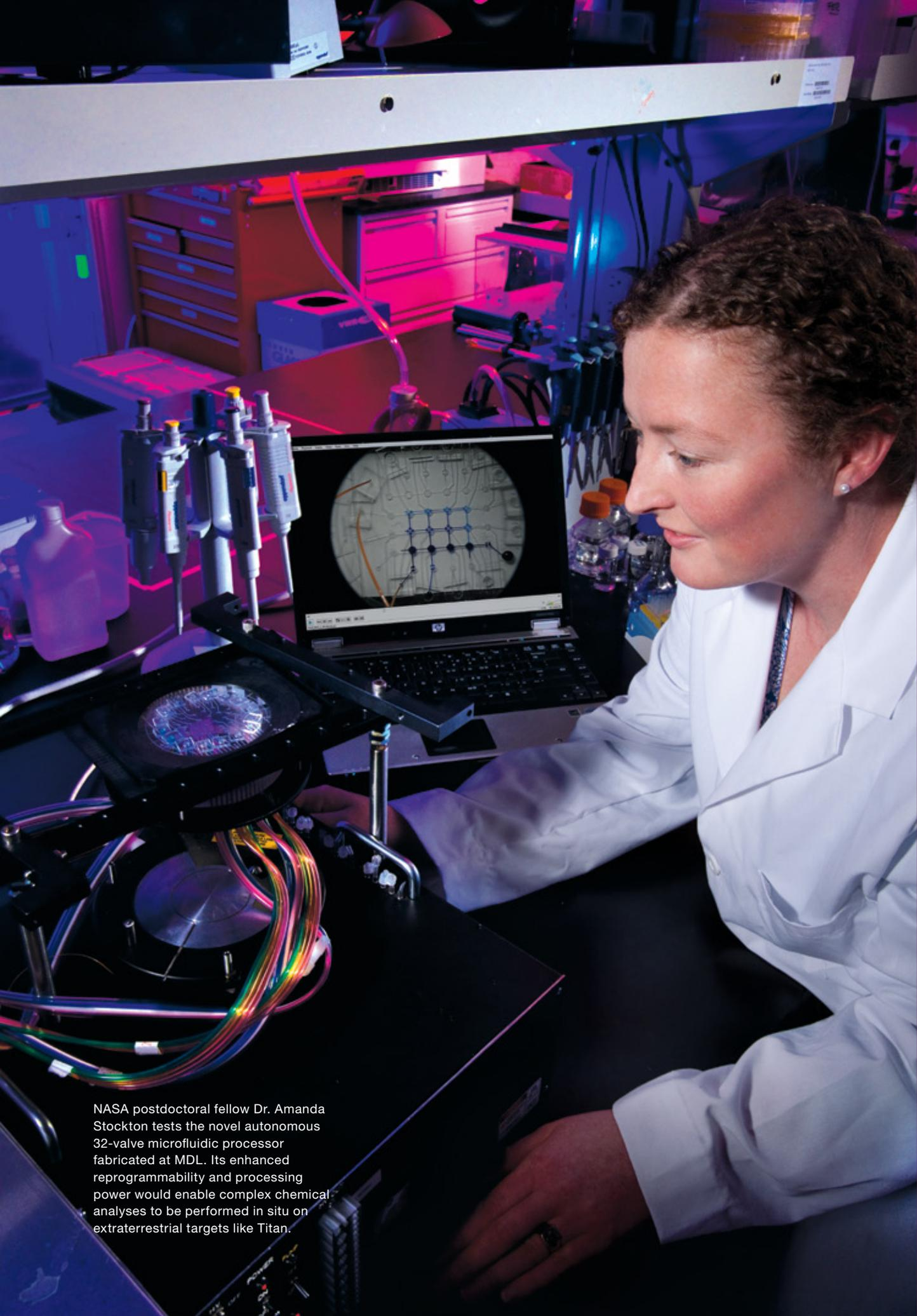
NASA postdoctoral fellow Dr. Amanda Stockton tests the novel autonomous 32-valve microfluidic processor fabricated at MDL. Its enhanced reprogrammability and processing power would enable complex chemical analyses to be performed in situ on extraterrestrial targets like Titan.
