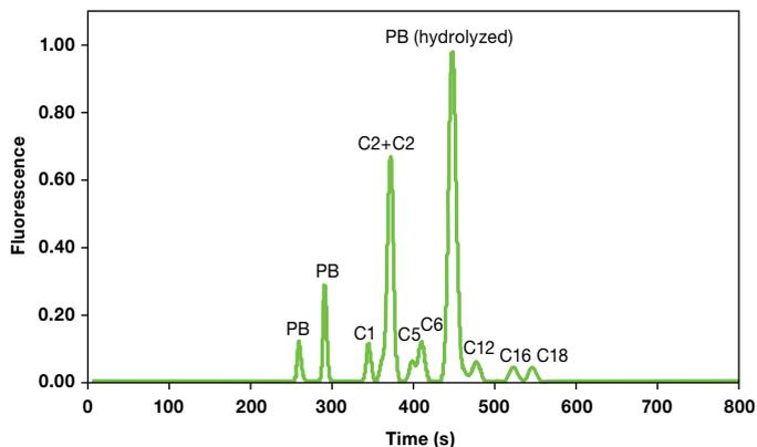
Analysis of a mixture of organic compounds, specifically amines with different carbon chain lengths (C1 to C18). They are dissolved in ethanol and detected on a lab-on-a-chip device. PB is Pacific Blue, the dye that attaches to the amines and makes them fluorescent.
