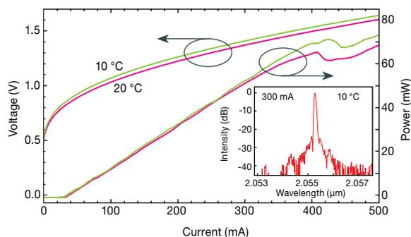
Above: Light-current-voltage characteristics of a laterally coupled DFB laser operating near room temperature. Inset: The single-mode laser emission spectrum at an operating current of 300 mA.
