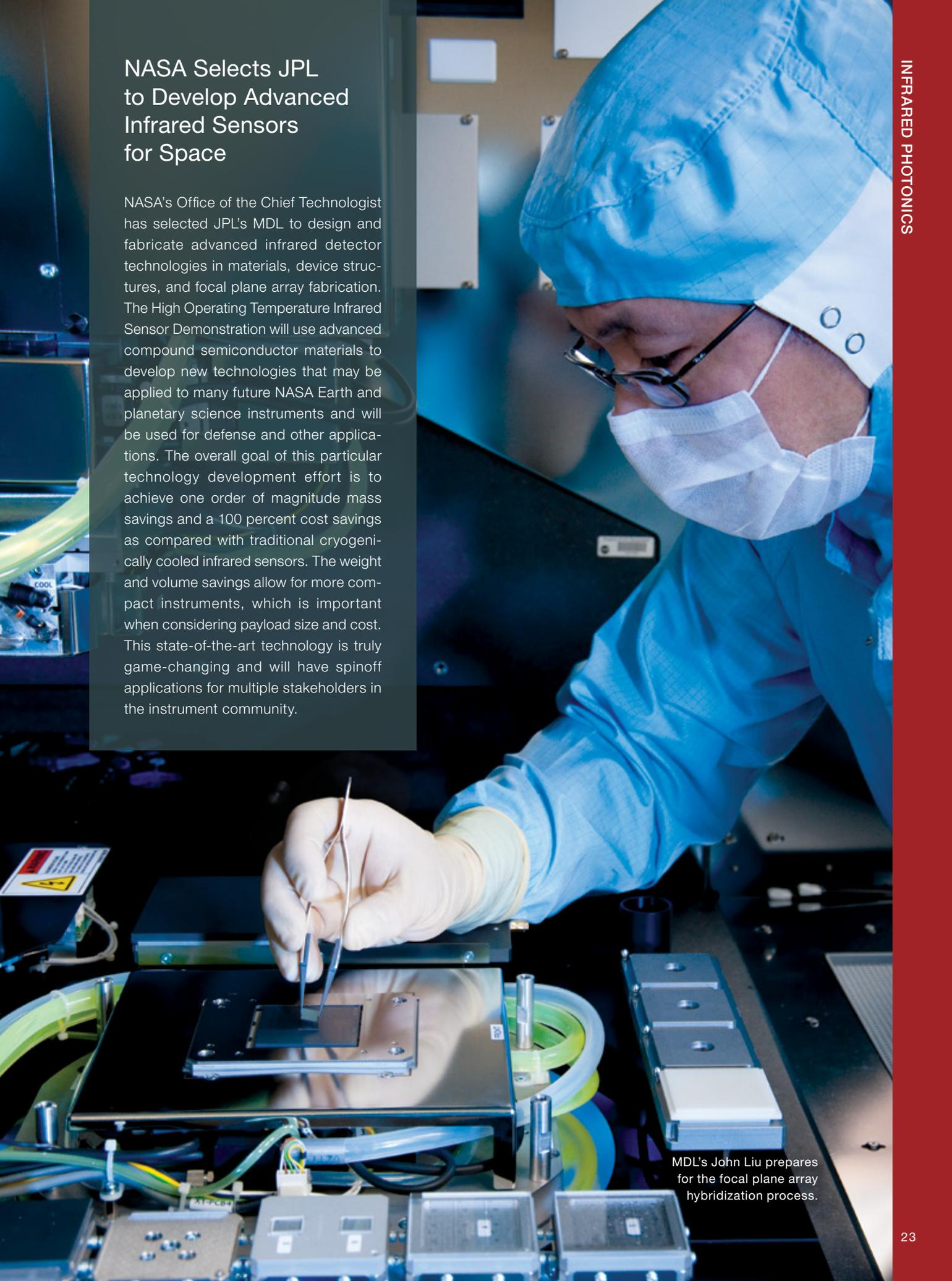
MDL's John Liu prepares for the focal plane array hybridization process.
