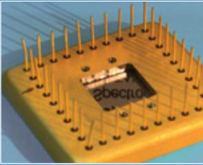
Left: A delta-doped low-energy electron detector was delivered for the LEES instrument on board the MICA sounding rocket.
