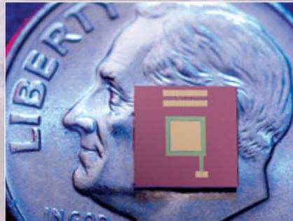
Above: The prototype CERES detectors consist of a large, thermally isolated silicon nitride membrane surrounded by roughly 1000 thermocouples. These thermocouples are composed of Bi-Sb-Te compounds and are the key to the high performance of the detector.
