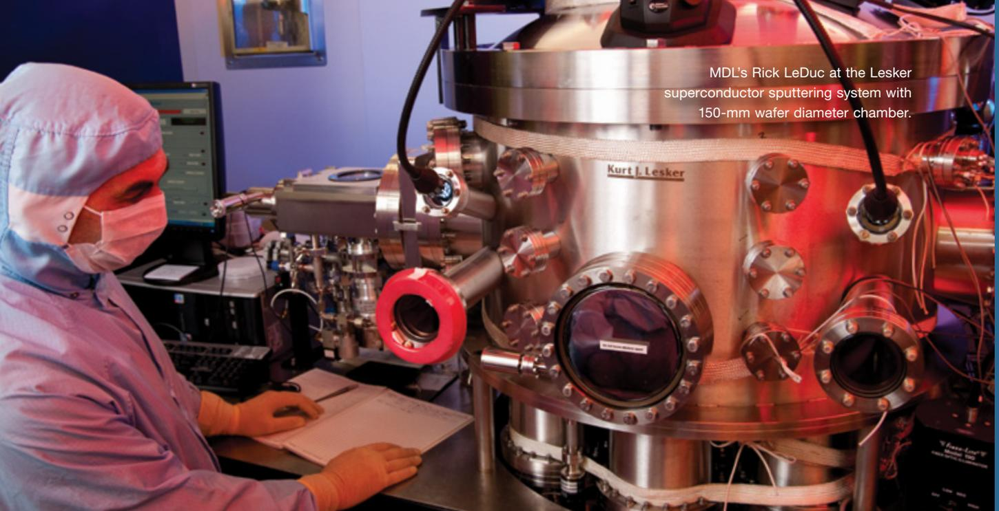
MDL's Rick LeDuc at the Lesker superconductor sputtering system with 150-mm wafer diameter chamber.
