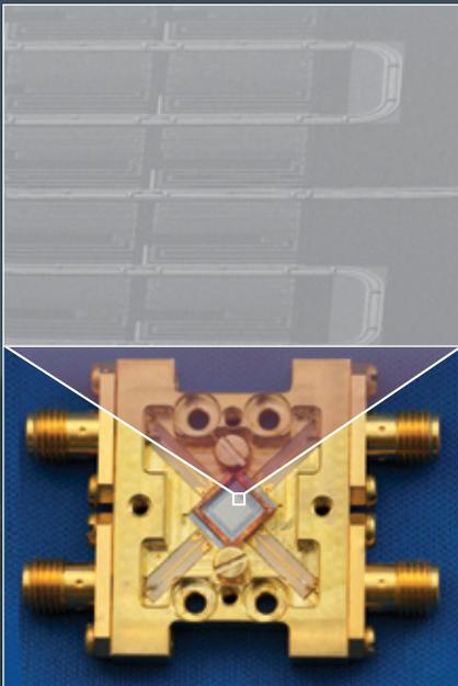
Above (top): Scanning electron microscope image of OLE MKID showing 10 of 1024 pixels and the microwave readout line. Each pixel is on a 100- $\mu$ m pitch and has a 0.5-mm resonator line spacing.
