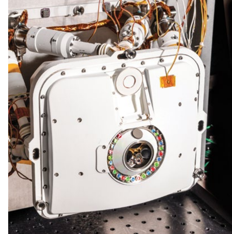
PIXL Instrument engineering model in test
