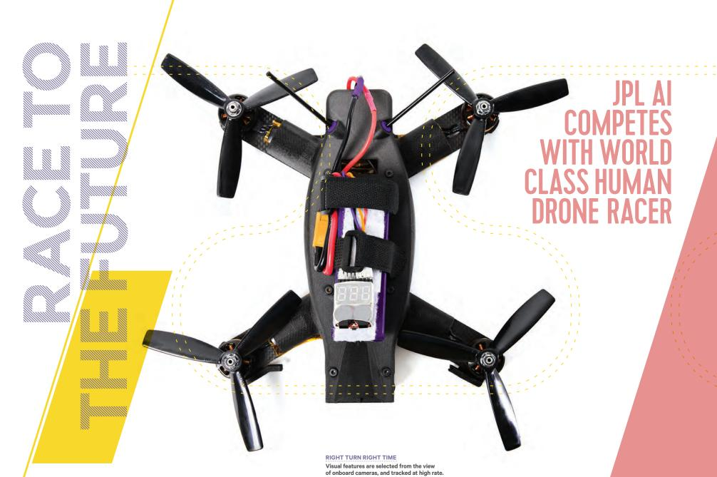
Visual reatures are selected from the view of onboard cameras, and tracked at high rat. The result is a versatile mobility platform that can navigate 3D terrain at high speed.
