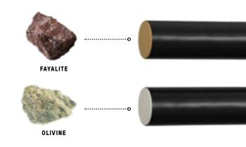
Ocean worlds relevant geological samples are used to coat the electrodes in a mineral paint (here, olivine and fayalite). Optimizing fuel cells for science requires different materials and processes than optimizing them for energy generation.
