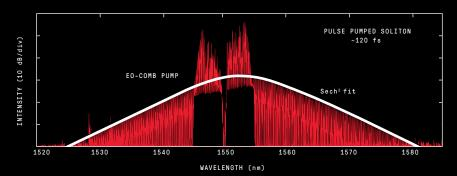
Figure showing a broad spectrum of uniformly spaced frequency comb lines generated by pulse-pumping a soliton microcomb
