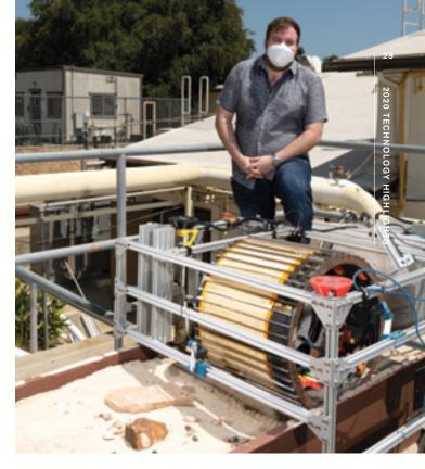
The Barefoot Rover testbed was utilized to train machine learning algorithms on different materials, surface conditions and material hydrations. Here, Jack Lightholder poses with the testbed.
