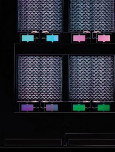
Left: A microscope image of a small array of antenna-coupled thermal kinetic inductance detectors (TKIDs), fabricated on a common chip. The four integrated antennae are the large squares dominating the image, while pairs of TKIDs sit under each antenna.
