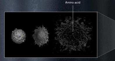
On the cover is the computer simulation of arginine amino acid encased in a 6.4 nm ice grain survives a simulated hard impact at 5 km/s. This provides quantifiable insight into future instrument design and mission parameters for hypervelocity sampling of biosignatures from ocean world atmospheres and plumes.
