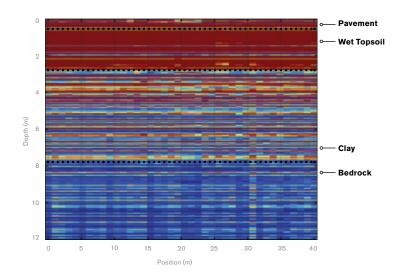
Prototype ground-penetrating radar product measuring the sub-surface beneath a road at JPL.
