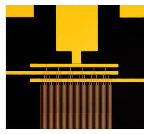
An optical image of a tunable surface acoustic wave transducers used for tunable-pitch diffraction gratings.
