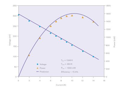
This graph shows the 15 percent thermal-to-electric conversion efficiency in an RTG enabled with JPL's new Zintl phase thermoelectric designs. Current designs have about six percent efficiency. The increase in efficiency can result in longer, more effective deep space missions.
