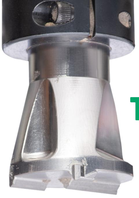
A close-in view of the abrading drill bit, which can characterize the firmness of soil surfaces before the rover drives across them.
