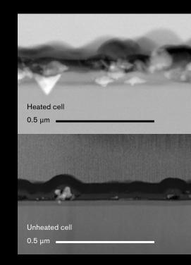
Top: Cross-sectional view of the solar cell, while heated, looking at the interface between the anti-reflective protective coating and the cell's surface. Silver melt droplets form, extending deep into the semiconductor layer.
