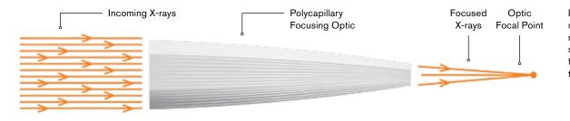
Incoming X-rays are focused by a bundle of millions of small glass capillaries, shaped to redirect the X-rays' grazing incidence to a much smaller focal spot. In this way the effective field-of-view of an X-ray detector, positioned at the focal spot, can be significantly increased.
