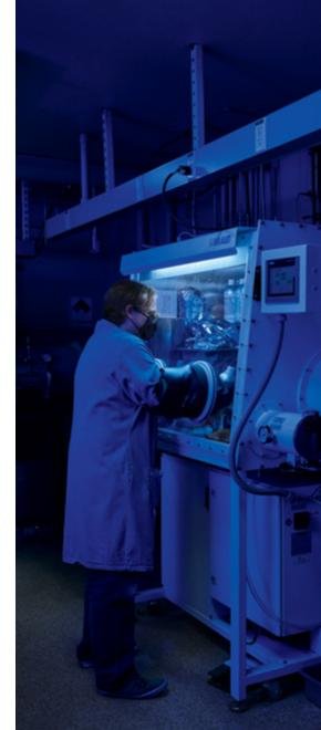
Custom low temperature Li-ion battery electrolytes are prepared in environmentally controlled glove boxes
