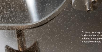
Counter-rotating rasps cut through surface material throwing sample material into a guide that directs it into a sealable sample collection cup.
