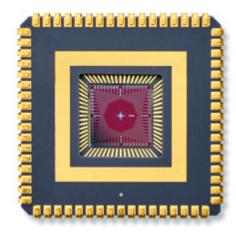
64-element SNSPD focal plane array developed at JPL for the NASA DSOC project
