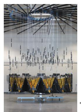
The Starshade inner disk testbed unfolds at Tendeg in Louisville Colorado. This testbed was used to demonstrate the deployment accuracy needed for Starshade concepts.
