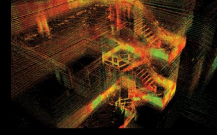
3D map generated by NeBula while traversing four flights of stairs. The map was created in real-time using onboard computation and software.
