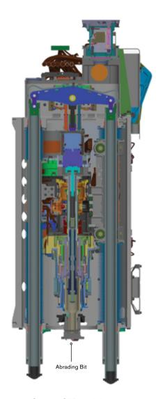
Cutaway CAD rendering of the entire drill system.
