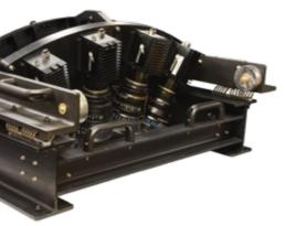
The QUAKES-I instrument (Quantifying Uncertainty and Kinematics of Earth Systems Imager) is a structurefrom-motion sensor developed by JPL to produce high resolution 3D terrain data products for the scientific community. The instrument consists of two sensor suites
