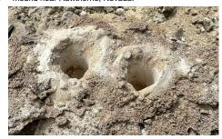
Bore holes and tailings produced by our M2020 analog coring bit.
