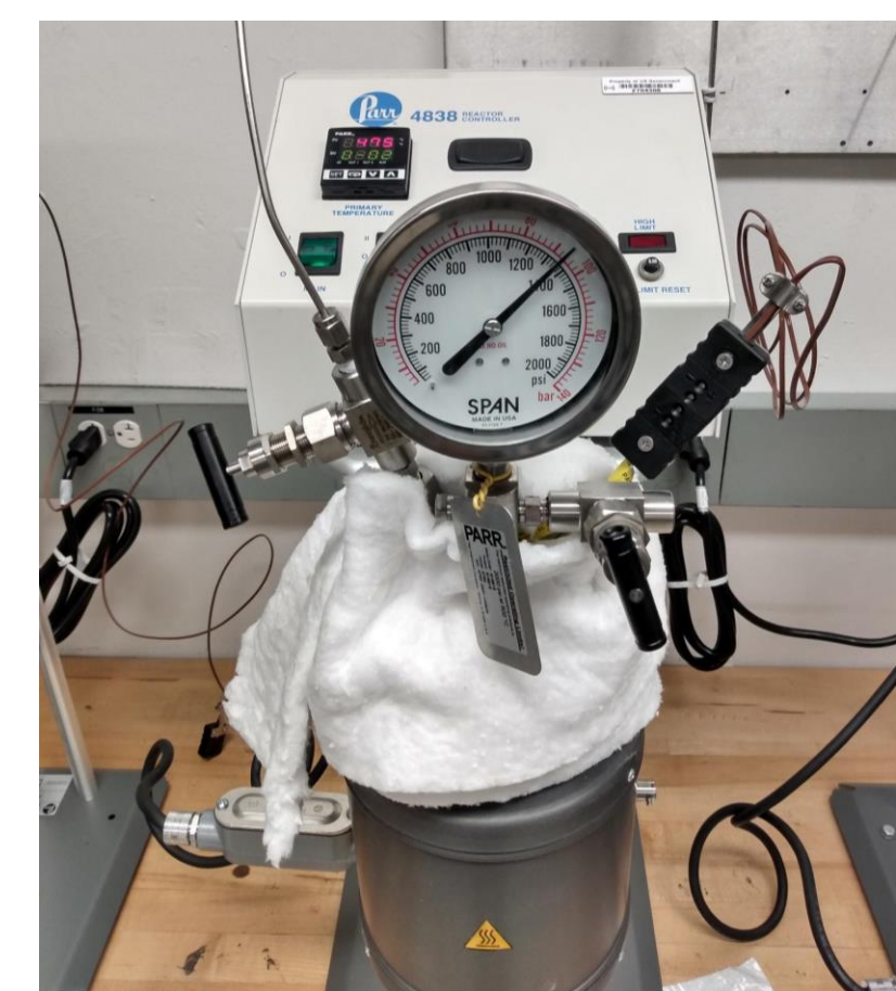
Figure 4: L) Photo of magnetite mineral after a 5 day weathering experiment (450 °C, 92 atm) in the JPL Venus reactors. R) one of the five operational Venus reactors in the JPL Planetary Geochemistry Simulation Facility
