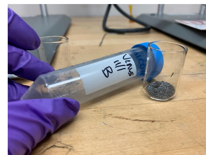
Figure 4: L) Photo of magnetite mineral after a 5 day weathering experiment (450 °C, 92 atm) in the JPL Venus reactors. R) one of the five operational Venus reactors in the JPL Planetary Geochemistry Simulation Facility
