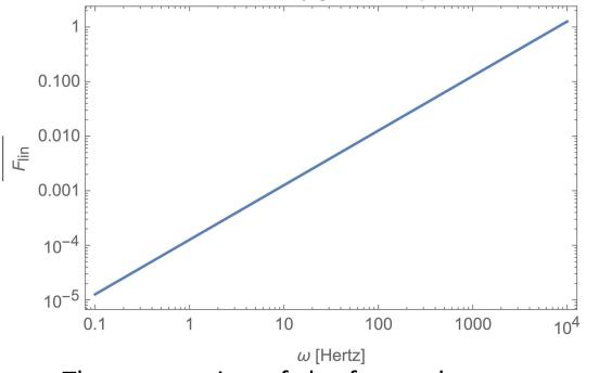
The attenuation of the forces due to stray magnetic gradients for a spin-zero trap
