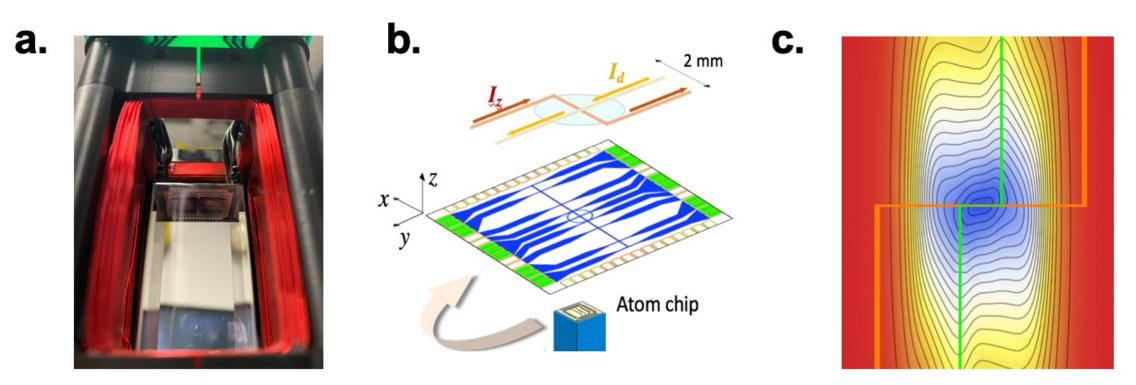
An atom chip located at the top of a dual-celled vacuum chamber (a.) is capable of forming a trap for neutral atoms by running currents through micro-wires on the semiconductor chip. The "z-d" planar geometry (b.) produces a [1.0, 1.0, 0.2] kHz trap for Rb atoms in the mf=2 state. A simulated atom chip trap shown here (c.) uses a BECCAL-like chip design.
