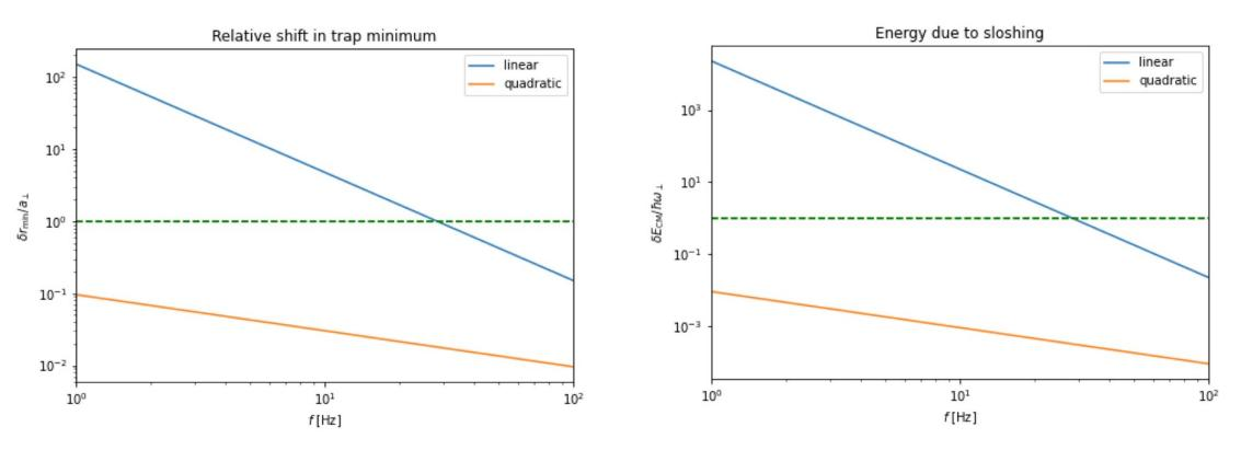
For a spin-zero trap (quadratic) in the presence of a 0.1 G/cm gradient, the left plots show the trap's relative displacement is smaller (and therefore more stable than) a standard (linear) trap. The right plots show the heating or equivalent energy that would be imparted to a sloshing mode due to this physical shift of the trap bottom during a trap decompression. This advantage of the quadratic-Zeeman trap over the linear case is further magnified at lower trap frequencies.
