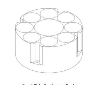
8-cell (2-battery) cassette, to be 3-D printed in polyme
