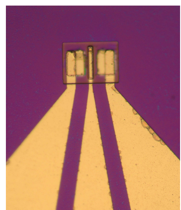
Figure 3: (a) 40 \mu\text{m} fabricated QWIP device. (b) The frequency measurement of the second round of fabricated devices with the probe station.
