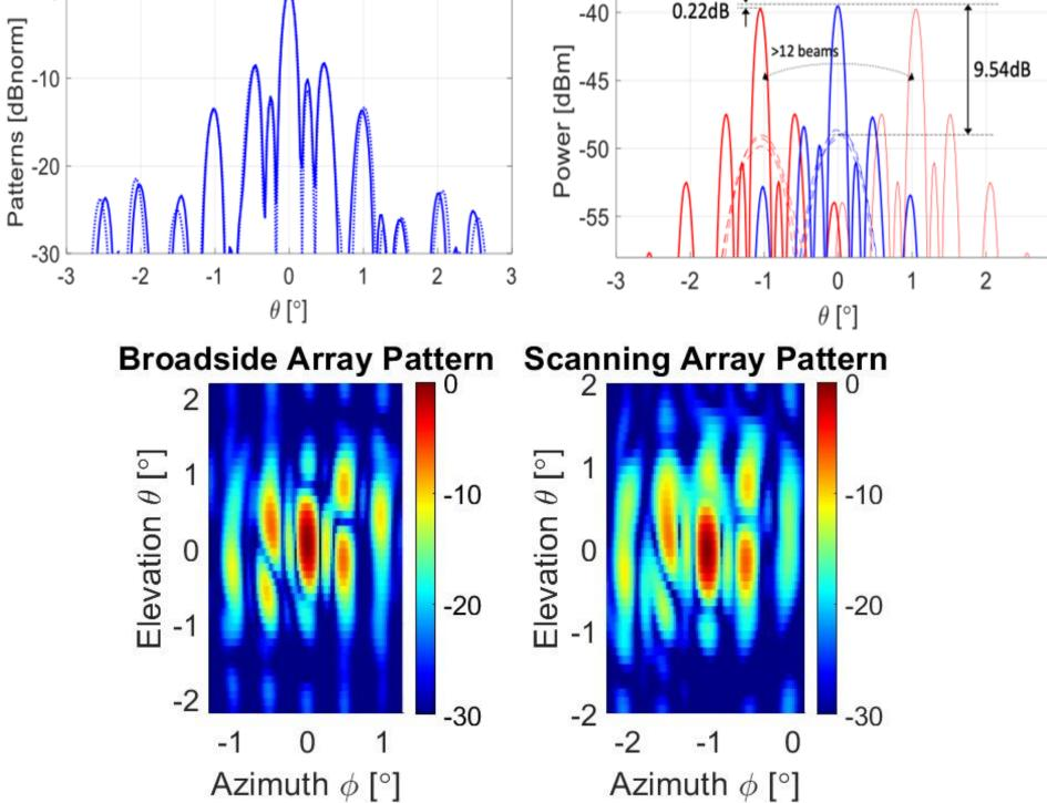
Measurements show excellent agreement with simulation, resulting in 9.5 dB higher power density and the potential for more than 12 beam widths of electro-mechanical steering capability.
