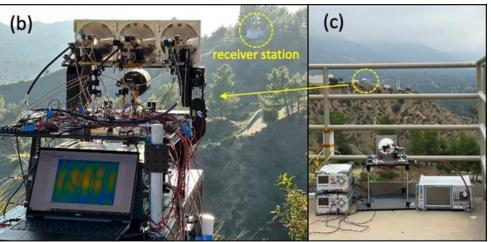
Photographs of three-element coherent-array powercombining and beam-steering tests at the JPL mesa.
