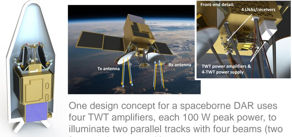
used to generate a coherent, power-combined radar beam that is steerable by simultaneously deflecting low-mass subreflectors of each antenna array element.
