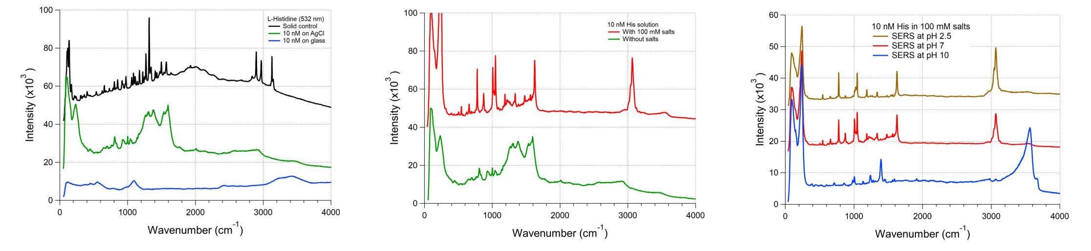
Demonstration of SERS activity on the detection of amino acid, where droplets of 10 nM L-histidine solution are deposited on the AgCI substrate. SERS effect is evident compared to the spectrum on the uncoated slide. Addition of a putative Europa brine (Na, Mg, Cl,  $SO_4$ ) does not suppress SERS activity. On the contrary, the presence of salts can be beneficial to SERS by significantly enhancing the SNR of the spectrum (top trace).
