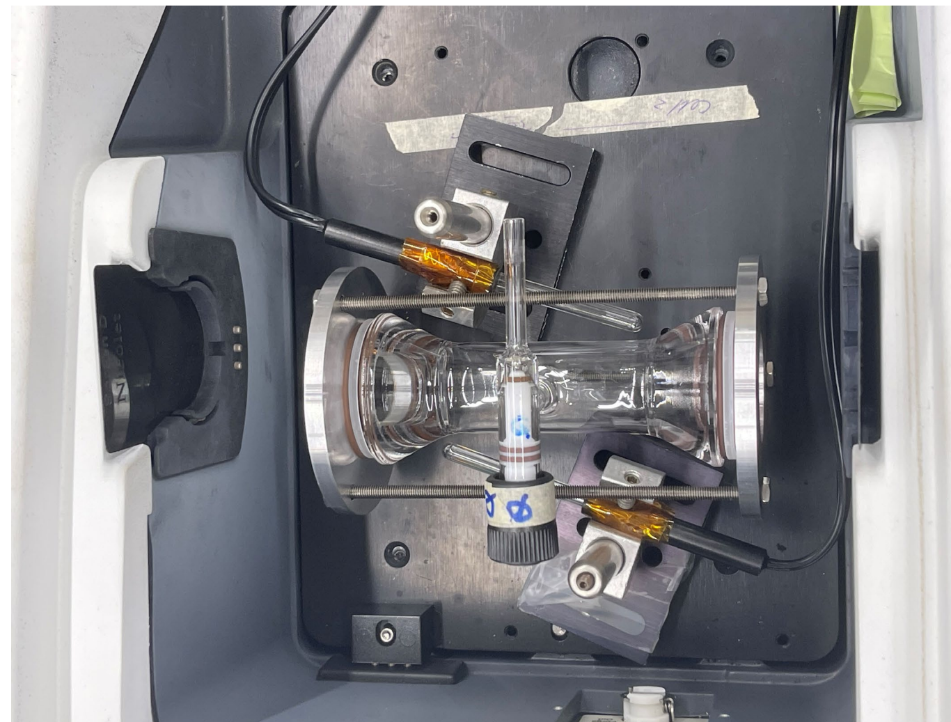
Fig. 3. Photolysis of \text{CO}_2 in a gas cell using two Hg lamps
