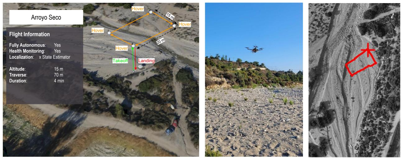
Fully autonomous mission execution demonstration on Earth demonstrator UAS. Left: Mission plan; Middle: Earth demonstrator UAS executing the mission; Right: Flight track (using onboard GPS)
