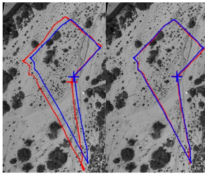
State estimation with map-based localization (MBL) using a keypoint-
