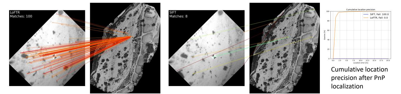
Significant scale change: Flight at 12m altitude, map with HiRISE resolution (25cm/pix)
