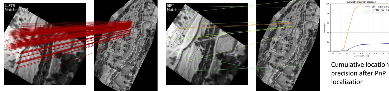
Significant lighting change: Flight at 100m altitude, map created in evening (5:30pm) with HiRISE resolution (25cm/pix), flight in the morning.
