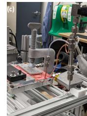
(a) A schematic demonstrating a possible change in design philosophy for additively manufactured LHP evaporators. (b) A schematic of the test LHP system. It is designed such that the evaporator can be rapidly swapped out while keeping the rest of the system constant. (c) A picture of the test setup during operation. (d) A picture of six AM aluminum LHP evaporators. (e) A plot showing operation of the LHP with 20W input heat.
