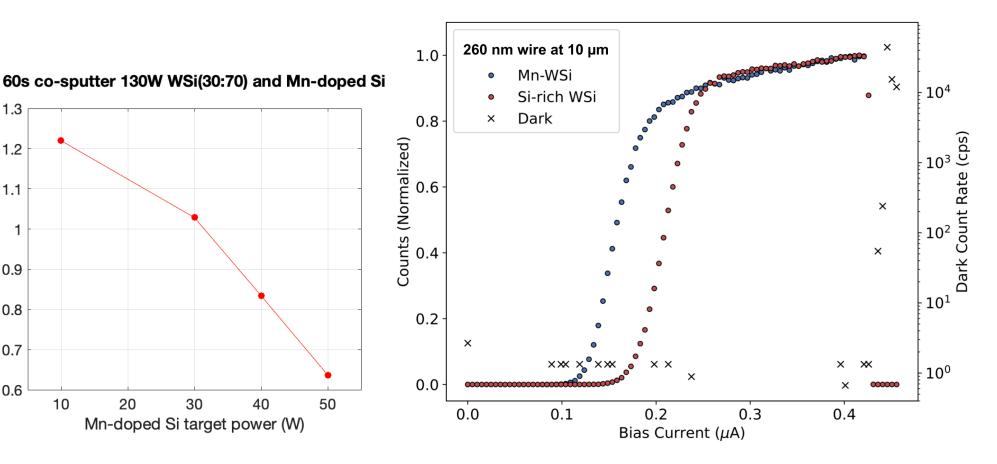
Photo-counts vs. bias current for 260nm-wide nanowires fabricated from the Si-rich WSi and Mn-doped WSi films. The detectors show saturated IDE despite their wider width. The Mn-doped detector has an enhanced IDE plateau.
