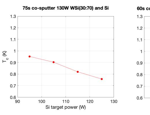
Critical temperature vs. sputtering power for Si-rich-WSi (left) and Mn-WSi (right) thin films. The films are produced by cosputtering with a W30Si70 target at a fixed power of 130 W. T<sub>c</sub> decreases with increasing Si and Mn-doped Si content, signifying a smaller energy gap and higher sensitivity to lowenergy photons.
