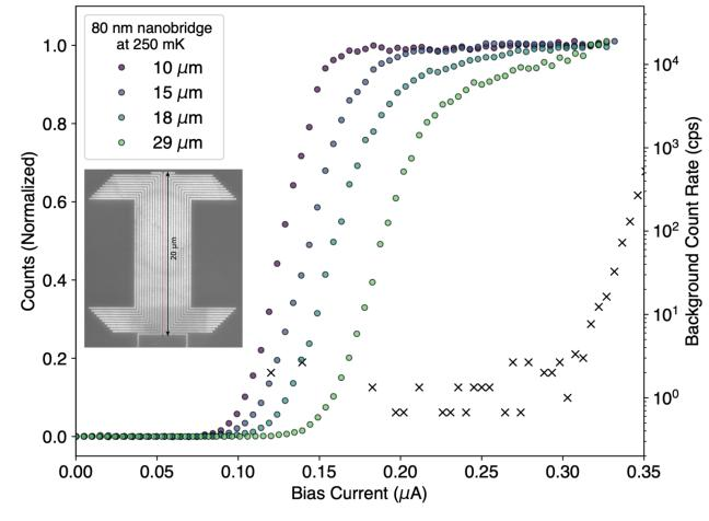
80nm-wide nanowire device measured with a filtered blackbody source at wavelengths from 10 to 29 µm. The detector exhibits saturated internal detection efficiency (IDE) vs. bias current, indicating that every absorbed photon produces an output pulse.
