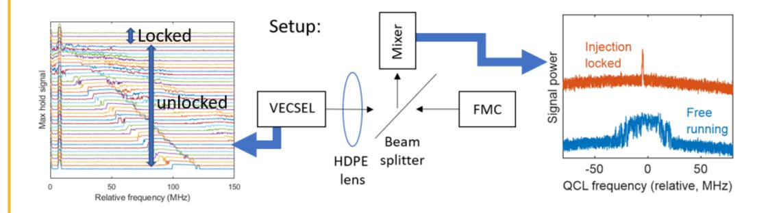
Center: A simplified diagram of the injection locking experiment. The QCL
